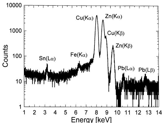
Fig. 3. Fluorescence spectrum of a metal alloy of known elemental composition (Cu–58%, Zn–40%, Pb–1%, Fe–0.15%, Sn–0.20%, ...).
