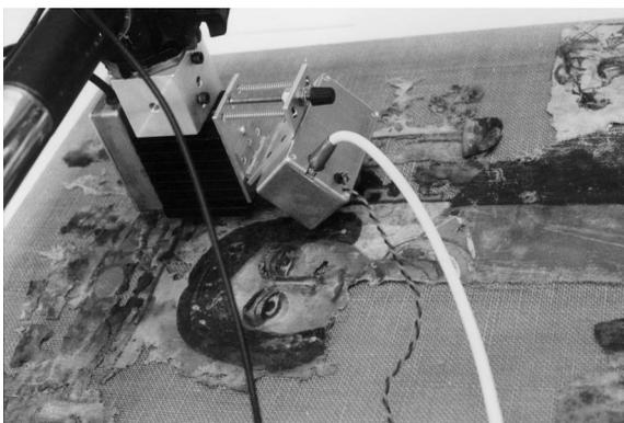
Fig. 1. The portable XRF spectrometer during a measurement on an Egyptian linen.
