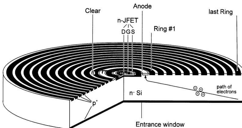
Fig. 2. Structure of the SDD with an integrated JFET.
