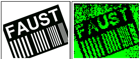
Figure 8: a) FAUST-MTF test chart as placed on the hexagonal pixel DEPFET matrix (left) b) recorded shadow image in binary readout using 6 keV X-rays (right).
