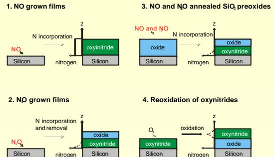
Figure 2: Production methods for oxynitrides: 1. Growth in pure NO, 2. Growth in pure N<sub>2</sub>O, 3. Annealing of oxides in NO or N<sub>2</sub>O, 4. Reoxidation of oxynitrides.
