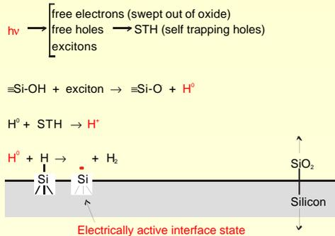
Figure 1: The hydrogen-model for radiation induced interface states: atomic hydrogen is formed by the reaction of excitons with OH-groups. Atomic hydrogen near the interface reacts with Si-H-bonds and forms an interface state. Atomic hydrogen formed in the oxide itself reacts with self trapped holes (STH) and forms a proton. The proton drifts to the interface and also forms interface states.
