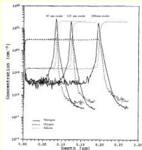
Figure 3: SIMS-measurements with oxynitrides of different thicknesses. The samples were produced by a two hour annealing of oxides in NO at 1050°C after oxidation at the same temperature. Noticeable is the sharp peak of nitrogen at the interface silicon-oxide.
