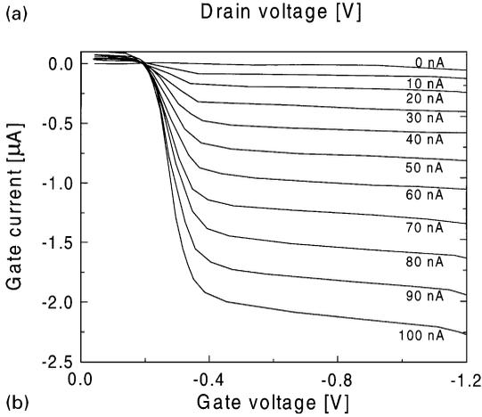
Fig. 3. (a) Characteristic curves of the nJFET with the BJT emitter grounded. (b) Characteristic curves of the reset BJT. In (b) the voltage applied to the gate of the JFET represents the potential difference between the collector and the emitter of the BJT. While tracing the BJT curves, the nJFET was operated with  $V_D = +3$  V.
