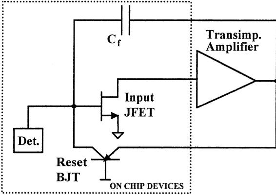
Fig. 1. Schematic representation of the charge amplifier showing the elements integrated on the detector chip: the input nFET, the feedback capacitor and the reset BJT.
