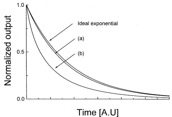
Fig. 5.  $\delta$ -response of the charge amplifier with  $C_f = 60$  fF and a BJT in the feedback loop. The figure compares the response - curve (a) - to a small signal ( $Q/C_f = 0.2V_T$ , equivalent to the signal from an  $^{55}\text{Fe}$  source) and the response - curve (b) - to a large signal ( $Q/C_f = 2V_T$ , equivalent to the signal from a 60 keV line) with the ideal exponential decay having  $R = V_T/I_{leak}$ .
