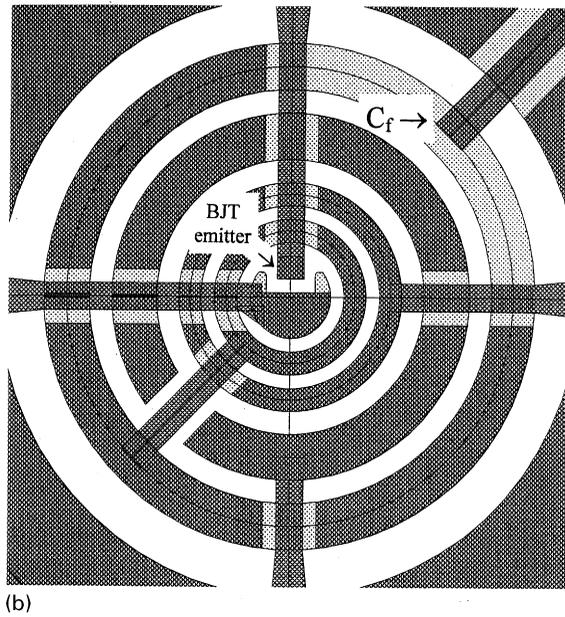
Fig. 2. (a) Schematic cross section of the on-chip electronics. (b) Top view of the anode region and on-chip electronics of the circular drift detector. The four rings are, from the outer to the inner, the anode, the isolation guard, the drain and the gate. In the center the source and the small BJT emitter are visible. The diameter of the outer ring (anode) is 110  $\mu\text{m}$ . Energy and doses of the implants are the same as reported in Ref. [1].
