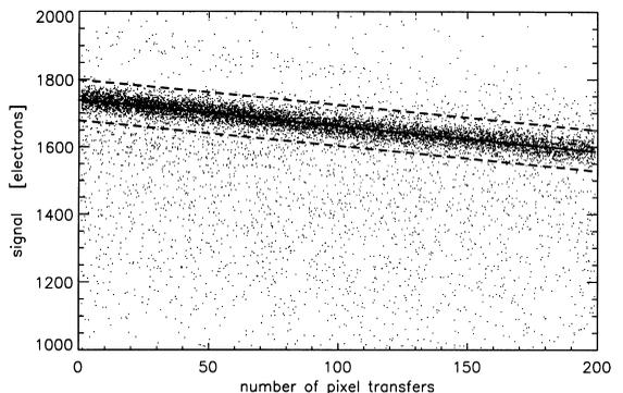
Fig. 3. Signals (dots) in dependence of the transfer length. The signals within the dotted lines were used for analysis. The solid line represents the mean charge loss.
