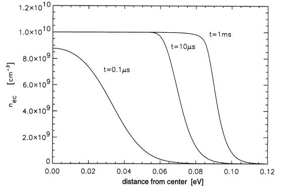
Fig. 1. Calculated density of captured electrons.
