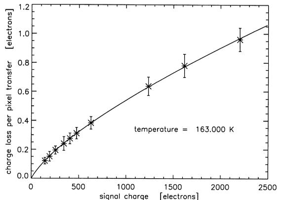
Fig. 4. Dependence of the transfer loss from the signal charge.  $\Delta t \geq 0.1 \text{ s}$  and  $T = 163 \text{ K}$ . This is equivalent with an empty traps condition. The solid line is the resulting charge loss calculated from the model. The employed parameters are based on a least-squares fit of the model to the data (star-shaped symbols with error-bars).
