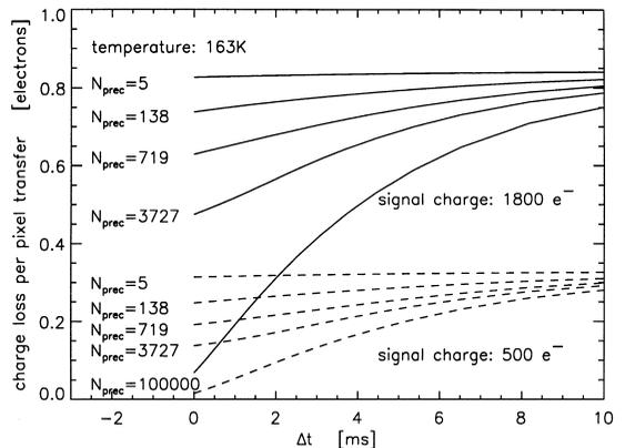
Fig. 2. Dependence of the charge loss per pixel transfer for a set of two signal charges of 1800 and 500 electrons.  $N_{prec}$  is the number of electrons in the preceding signal.
