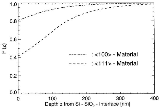
Fig. 3. Collection function for  $\langle 111 \rangle$ - and  $\langle 100 \rangle$ -material; the parameters are the same as in Fig. 2.
