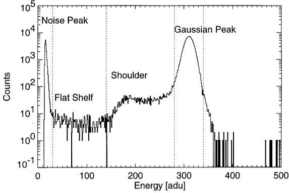
Fig. 1. A typical spectrum, taken at 1400 eV synchrotron radiation; one can well distinguish between the Gaussian part, the low-energy shoulder and the flat shelf. Due to the event threshold, the noise peak is only partially recorded and therefore not centered around 0 eV.
