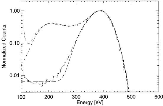
Fig. 2. Two examples of fitted spectra for different detector materials: dotted stepline: data for  $\langle 111 \rangle$ -material, short dashes: model fit with parameters:  $S = 0.42$ ,  $l = 106$ ,  $c = 1.16$ ,  $\tau = 96$ ; dash-dotted stepline:  $\langle 100 \rangle$ -material, long dashes: model fit with  $S = 0.81$ ,  $l = 50$ ,  $c = 1.0$ ,  $\tau = 93$ ; data were taken with a photon energy of 400 eV at the SX-700 monochromator at BESSY-I.
