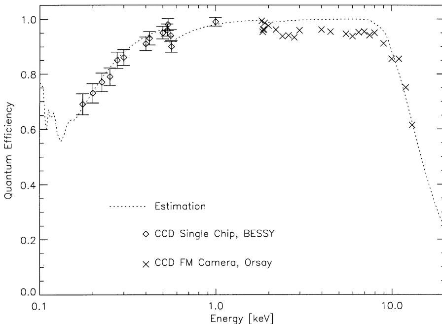
Fig. 4. Quantum efficiency of pn-CCDs measured at BESSY-I with monochromatic radiation (SX-700 monochromator), with preliminary data points for higher energies measured during the pn-EPIC flight model calibration at the Institut d'Astrophysique Spatiale (IAS) Orsay facility [12].
