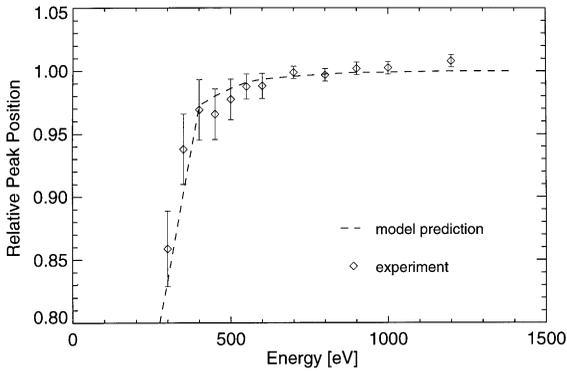
Fig. 5. Variation of peak position with energy: the relative peak positions (given in [adu/eV]) are normalized to the value at 1400 eV.
