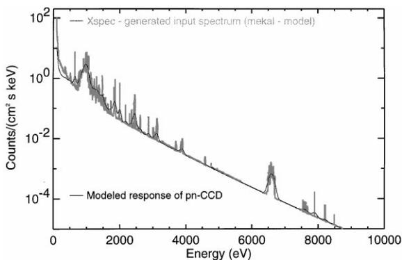
Fig. 7. As an example for a typical input spectrum, the model is applied to the simulation of an SNR (supernova remnant); neither filters nor telescope response is taken into account.
