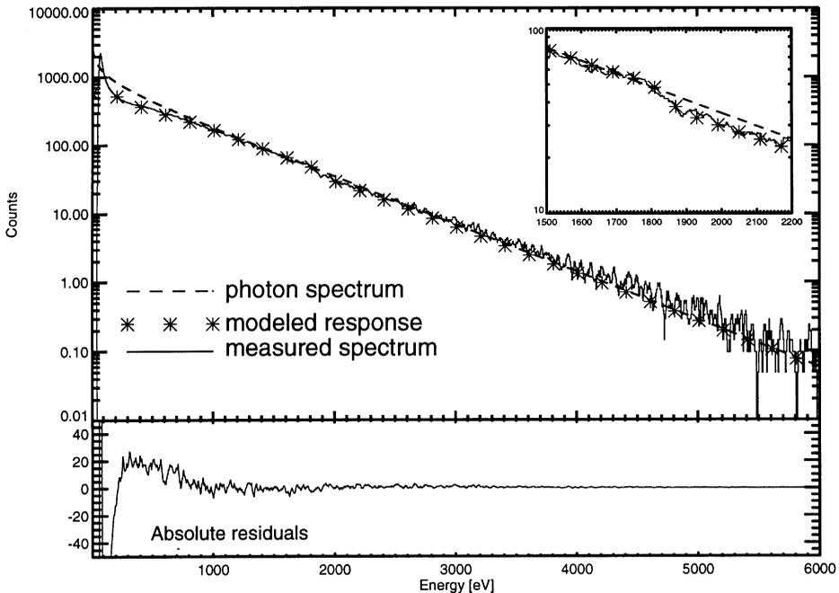
Fig. 6. Spectrum of white synchrotron light, together with the incident photon spectrum and the modeled CCD response. The inset shows details around the Si-K edge at 1839 eV.
