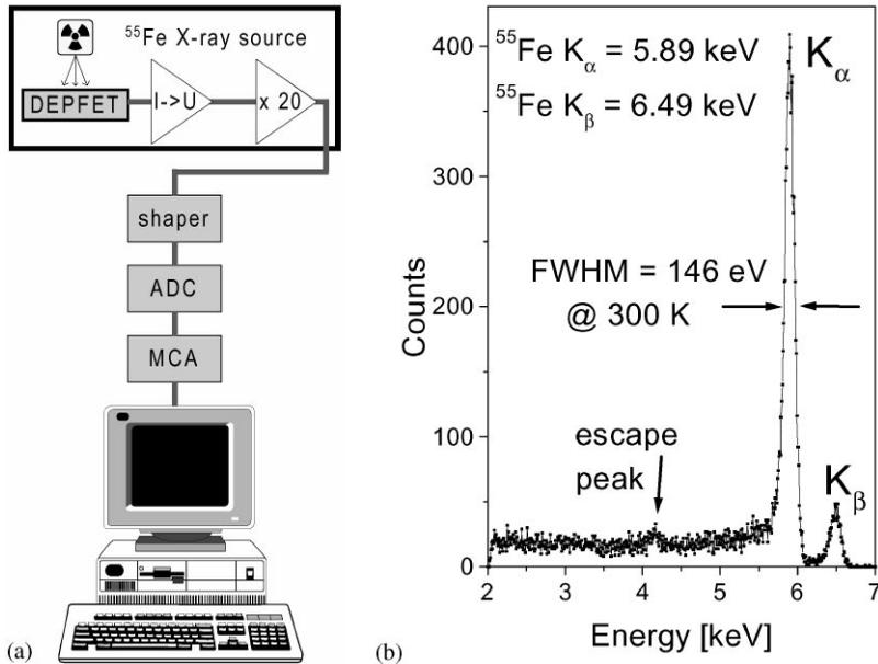
Fig. 4.  $^{55}\text{Fe}$  spectrum recorded with one DEPFET pixel; doing an energy calibration with the  $K_\alpha$  line and the  $K_\beta$  line and taking into consideration the Fano noise contribution, a noise value of  $9.5 \pm 0.1e^-$  at  $T = 30$  K and a shaping time of  $10 \mu\text{s}$  was determined.
