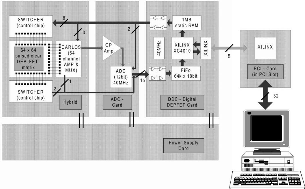
Fig. 3. DEPFET Bioscope system.
