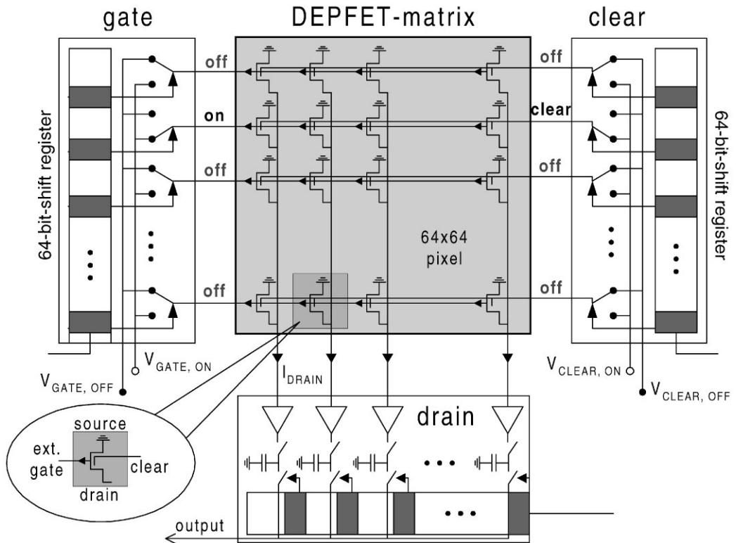
Fig. 2. Readout concept for the DEPFET pixel matrices.
