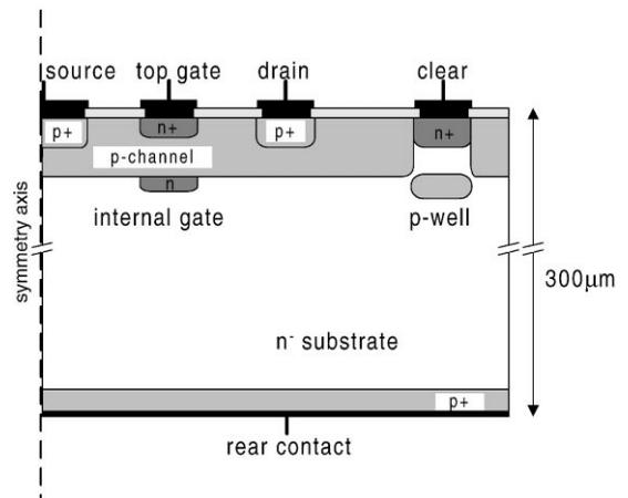
Fig. 1. DEPFET detector principle.
