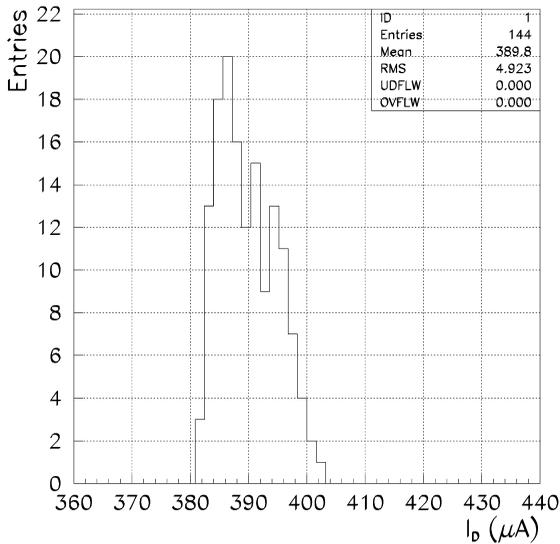
Fig. 5. Current variation within a  $16 \times 16$  DEPFET pixel matrix.
