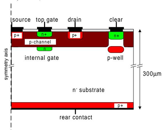
Figure 1: Cross section of an annular DEPFET pixel. The structure is symmetric along the symmetry axis shown.
