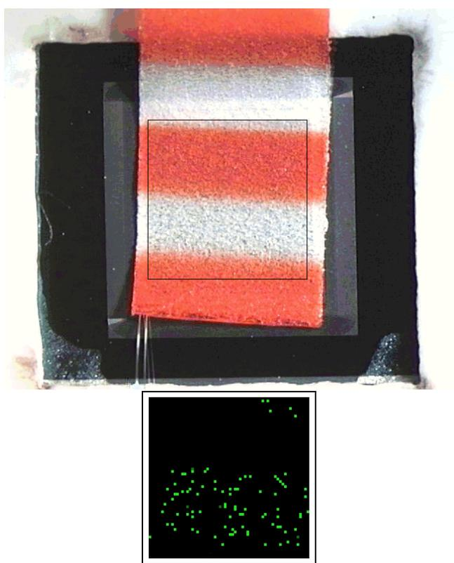
Figure 9: a) Photograph of a  $^3\text{H}$ -Microscale<sup>TM</sup> [11] placed on the entrance window of the DEPFET pixel Bioscope (top) b) screen shot of the online event display after several hours (bottom).
