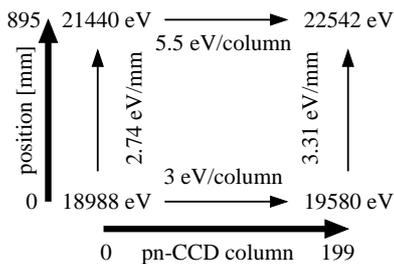
Fig. 3. Energy and dispersion at the pn-CCD detector as function of the column of the pn-CCD (lower horizontal scale) and position of the HOPG-crystal (left vertical scale). The quoted energies correspond to the indicated limits at the scales. Included are also the corresponding dispersions.
