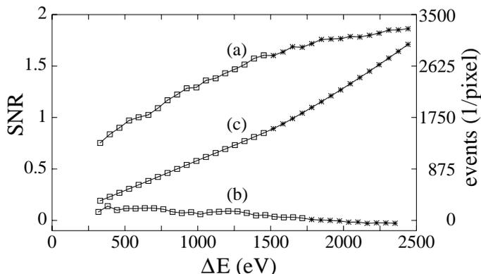
Fig. 9. SNR as derived from 416 pixels for a domain (a) covered and (b) not covered by the molybdenum sample foil. Curve (c) represents the number of photons in the energy interval  $\Delta E$ . Squares ( $\square$ ) indicate symmetrical fit intervals with respect to the K edge, asterisks (\*) asymmetrical ones.
