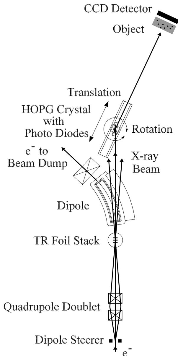
Fig. 2. Experimental setup at MAMI
