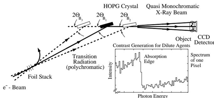
Fig. 1. Principle of the K-edge imaging system for contrast generation of dilute agents in an object. The inset shows the energy spectrum of a single pixel of the pn-CCD detector. The photon energy (abscissa) is defined by the position of the HOPG crystal at a translation stage.
