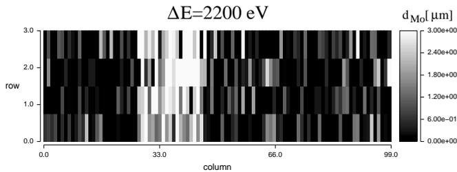
Fig. 8. Image of the phantom, shown in Fig. 4, with a  $272 \mu\text{m}$  thick copper bulk foil in a gray-level representation of the fitted molybdenum thickness. Negative molybdenum thicknesses are put to zero. Because of the poor counting statistics  $16 \times 2$  pixels are combined to a new pixel of  $2.4 \text{ mm} \times 0.3 \text{ mm}$  size.
