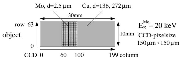
Fig. 4. Phantom used in the experiments located at a distance of 120 mm in front of the pn-CCD detector.
