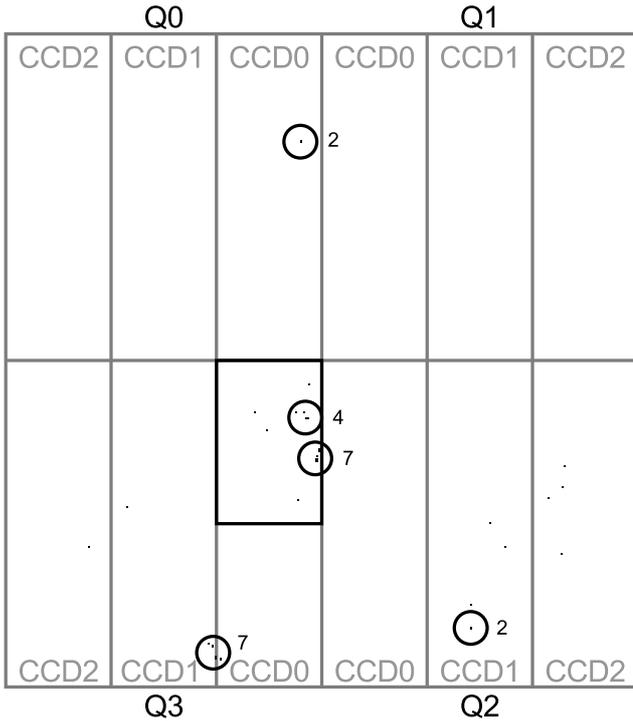
**Fig. 2.** Pattern of bright pixel distribution, occurring in orbit # 156. With the exception of one hit in quadrant 0, CCD0 all sources of bright pixels are located in an area with a radius of approximately 2 cm. The most severely hit device is CCD0 of quadrant 3. A time series of the framed area (CCD0, Q3) is shown in Fig. 4. The focal point of the X-ray telescope is located in the lower third of CCD0 in quadrant Q1.
