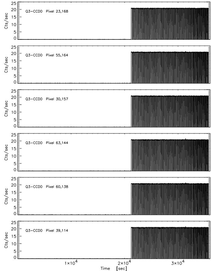
**Fig. 3.** Count rate increase in orbit # 156. Within one time resolution element, the 6 selected pixel of CCD0, quadrant 3, went into saturation, i.e. 21 event hits per second, which is  $1/0.0477$  counts per second in the large window mode.
