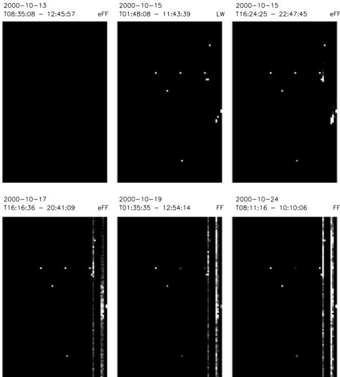
**Fig. 4.** Hit pattern of the suddenly appearing bright pixels in orbit # 156. The six images of CCD0 in quadrant 3 span a time of 11 days in total. The first (clean) image was made in the extended Full Frame mode (indicated as eFF), the second in the large window mode (LW), image 3 and 4 again in eFF and pictures 5 and 6 in Full Frame mode. The behavior seems to become stable after 4 days, to be seen at image 4 on October 17.
