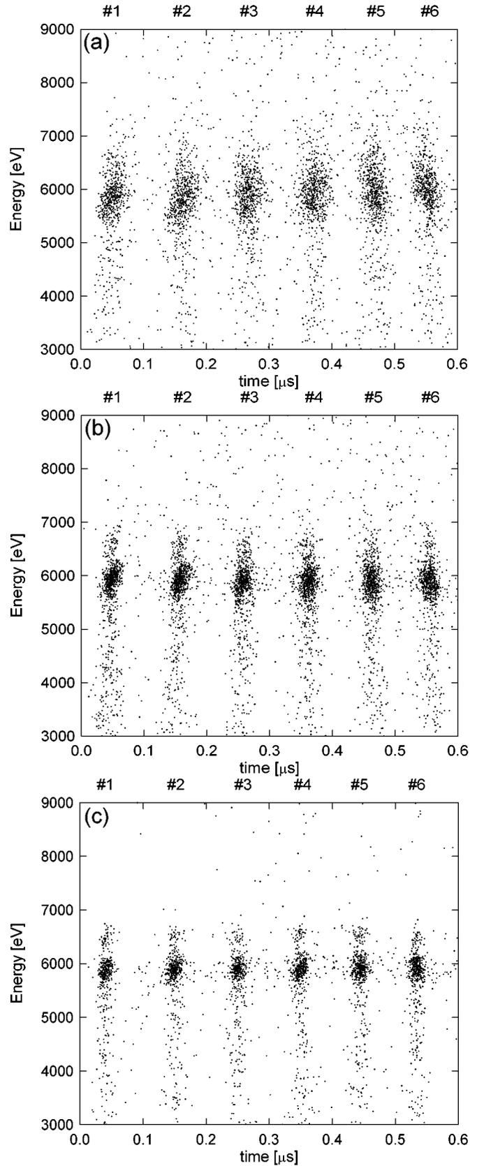
Fig. 2. Scatter plot energy versus drift time of the X-rays of a  $^{55}\text{Fe}$  source collected by a column of the CDD. The measurement was carried out at room temperature. The clusters have been labeled with the corresponding pixel numbers. (a) 10-kHz frame rate (integration time  $90\text{ }\mu\text{s}$ ), (b) 30-kHz frame rate (integration time  $30\text{ }\mu\text{s}$ ), and (c) 100-kHz frame rate (integration time  $9\text{ }\mu\text{s}$ ).
