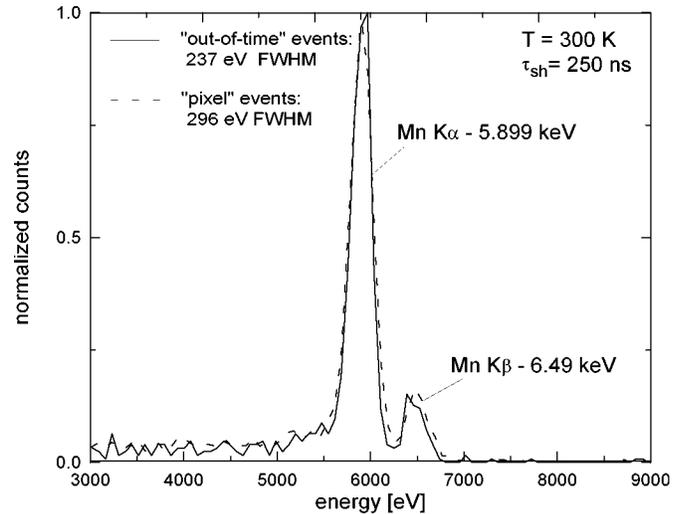
Fig. 6. Comparison of the distribution of the events of Fig. 5 along the energy and of the out-of-time events. The detector operating temperature is  $T = 300$  K and the shaping time is  $\tau_{sh} = 250$  ns.
