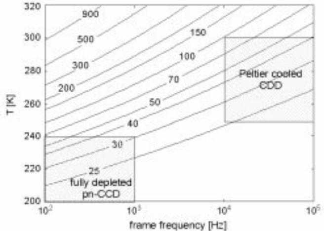
Fig. 8. Contour plot of the achievable energy resolution in terms of  $ENC$  as a function of the detector working temperature and of the frame frequency. The ratio between integration time and readout time is set equal to nine.
