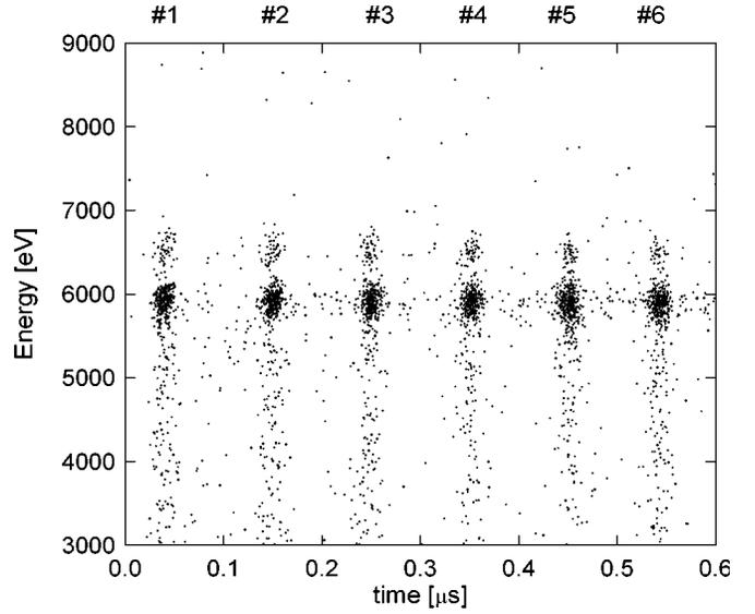
Fig. 5. Scatter plot energy versus drift time of the X-rays of a  $^{55}\text{Fe}$  source collected by a column of the CDD at 100-kHz frame frequency. The integration time was set to  $6.7 \mu\text{s}$  and the readout time to  $3.3 \mu\text{s}$ .
