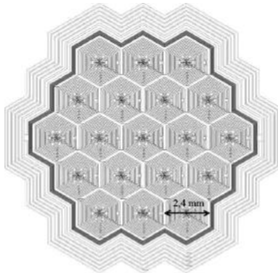
Fig. 1. Layout of the monolithic array of 19-SDDs. The detector side where the drift rings and the front-end JFET are integrated is shown. The scintillator is coupled to the opposite side of the detector.
