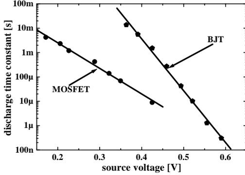
Fig. 5 Discharge time constant (related to leakage current) versus the DC output voltage when a MOSFET or a BJT is used as reset device. The relation is exponential for both systems, certifying that the MOSFET is operating in weak inversion regime. The difference in slope is due to the capacitive division between the gate oxide and the depleted bulk existing only in the MOSFET.
