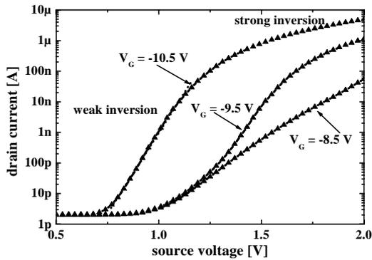
Fig. 3 Transfer characteristic curves of the reset MOSFET, obtained holding the MOSFET Drain at  $-1.5$  V.
