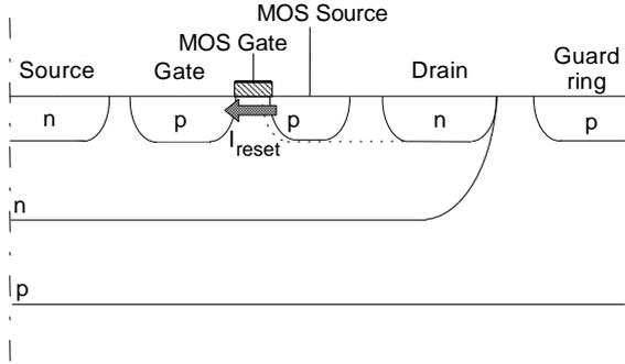
Fig. 2 Cross section of the inner part of the detector chip, taken radially through the reset device in the MOSFET version. The reset mechanism is obtained by the injection of holes from the MOSFET source into the JFET gate, directly connected to the detector anode.
