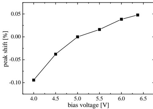
Fig. 6 Relative peak shift varying the  $p^+$  guard ring bias voltage. A variation of less than 0.15% in the peak position has been measured with respect to a variation of 2.5 V in the bias voltage.
