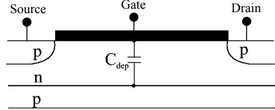
Fig. 4 Schematic view of a pMOSFET operating in weak inversion regime, showing the capacitive division responsible for the  $n$  factor.
