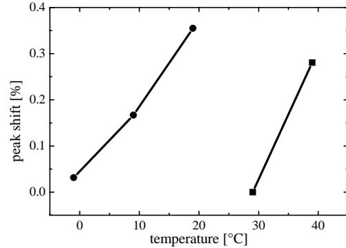
Fig. 7 Relative peak shift varying the operation temperature. A variation of 10 °C in the temperature causes a peak shift of about 0.2%. The two curves do not connect because the bias has been varied between the two experiments.
