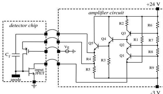
Fig. 1 Schematic of the charge amplifier. The amplifier circuit contains a transimpedance circuit that drives the feedback capacitance and the reset device integrated on the detector chip.
