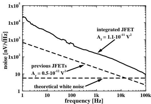
Fig. 9 Noise spectrum of the front-end nJFET. The high value of  $A_f$  is the main responsible for the ENC introduced by the electronics.
