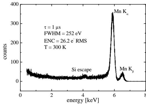
Fig. 8 Energy spectrum of a  $^{55}\text{Fe}$  spectrum acquired at room temperature at the optimal shaping time ( $1\ \mu\text{s}$ ). The measured resolution is 252 eV FWHM, corresponding to an ENC of 26.2 electrons rms. The silicon escape peak at 4.15 keV is also visible.
