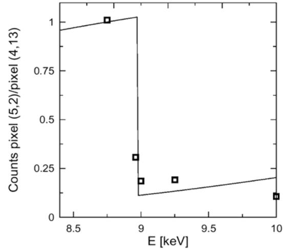
Fig. 7.: Normalized transmittivity of a 10  $\mu\text{m}$  thick Copper layer as a function of the energy around the K-edge. The squares are the experimental points and the line is the theoretical behavior.
