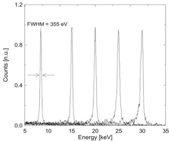
Fig.3.:Normalized-counts energy spectra of several energies in the range 8.5 keV – 30 keV, available at the SYRMEP beamline (Sincrotrone Trieste).
