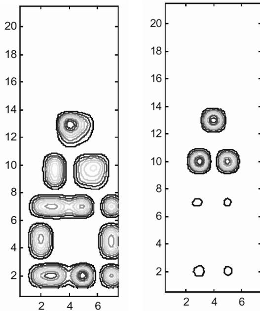
Fig. 6.: a) Scheme of principle of the phantom used to perform elemental absorption contrast imaging. b) Contour plot of the counts recorded by the CDD when the mask was irradiated with 8.5 keV X-rays (below the Cu K-edge). c) Contour plot of the counts recorded by the CDD when the mask was irradiated with 10 keV X-rays (above the Cu K-edge).
