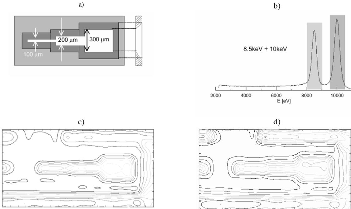
Fig. 5. a) Scheme of principle of the radiographed Silicon slit. b) Energy spectrum acquired by the CDD. The data of the irradiation with a 8.5 keV and the one of the irradiation at 10keV have been summed. The two energy windows used to calculate the images shown in c) and d) are indicated. c) Image of the slit irradiated with 8.5 keV. d) Image of the slit irradiated with 10keV.
