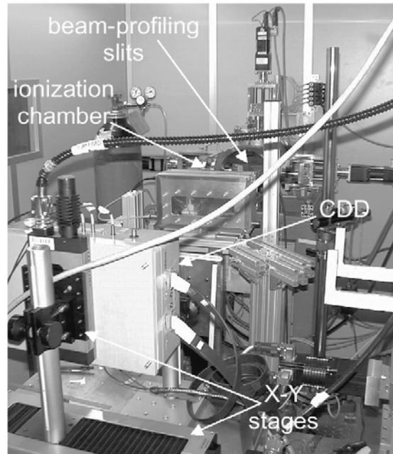
Fig.2.: Photo of the experimental setup at the SYRMEP beamline (Sincrotrone Trieste).
