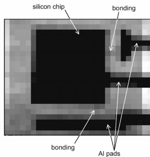
Fig.4: a.) Front view of the radiographed integrated circuit in a TO92 plastic package. b.) Radiography of the integrated circuit shown in a). The energy of the X-ray beam was set to 22 keV. The CDD was operated at 100kHz frame rate. The darker the pixel in the gray scale, the lower the number of counts in the pixel. The arrows indicate the bonding connections of the silicon chip to the metal pads.
