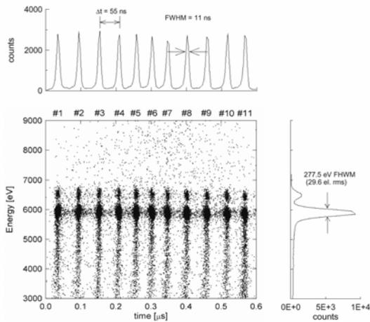
Fig.1.: Scatter plot energy vs drift time of the X-rays of a  $^{55}\text{Fe}$  source collected by irradiating a column of the CDD at 100 kHz frame frequency. The integration time was set to  $9\ \mu\text{s}$  and the readout time to  $1\ \mu\text{s}$ . The upper inset shows the distribution of the events along the time axis. The inset on the right end shows the total distribution of the event energies (i.e. the spectrum of the  $^{55}\text{Fe}$  source collected by all the pixels).
