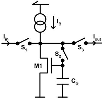
Figure 3. Basic principle of the current memory stage.
