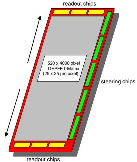
Figure 1. Conceptual design of one ladder of layer 1 of the DEPFET based vertex detector for TESLA.
