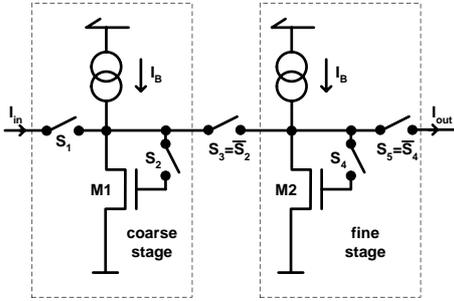
Figure 4. Basic principle of the two stage current memory cell.
