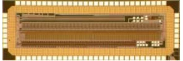
Figure 6. Photography of the 1.5x4 mm<sup>2</sup> prototype chip in 0.25  $\mu\text{m}$  radiation tolerant CMOS technology.
