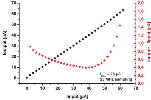
Figure 7. Linearity of the complete analog front-end (The points indicating the output current and the stars indicating the deviation between input and output current).
