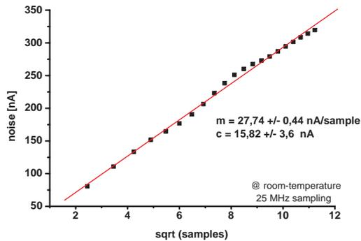
Figure 8. Total sampling noise as a function of the square root of the number of sampling steps.
