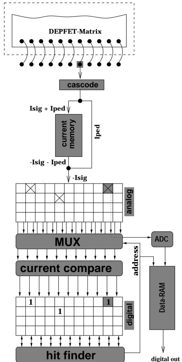
Figure 2. Basic Architecture of the readout chip. Partially only one channel is shown for simplicity.
