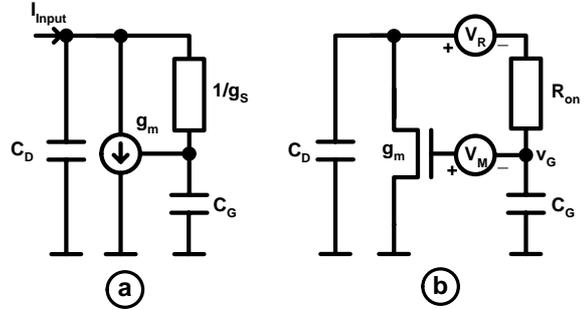
Figure 5. Equivalent circuit of the current memory cell during the charging phase (a), Circuit used for the noise analysis (b).
