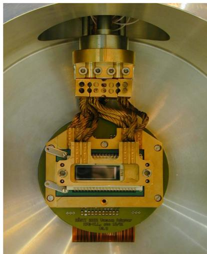
Fig. 6. Focal plane pn-CCD detector as mounted inside the CAST telescope. The Au-plated cooling mask surrounding the rectangular CCD chip in the center is connected to the cold finger of a Stirling cooler on top of the detector chamber. Electrical connections to the printed circuit board behind the CCD chip are provided via the flexlead leaving the chamber at the bottom. The internal Cu/Pb shield surrounding the detector has been removed.
