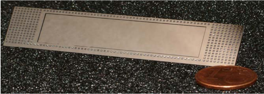
Figure 4. A silicon sample thinned down from 300 \mu\text{m} to 50 \mu\text{m} using the wafer bonding technique. A perforated frame has been left over to ensure mechanical stiffness.
