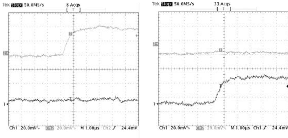
Fig. 9. Preamplifier signals measured on two contiguous channels. When one of the two channels is hit by a  $^{55}\text{Fe}$  signal, no noticeable cross-talk signal is detected by the other channel.
