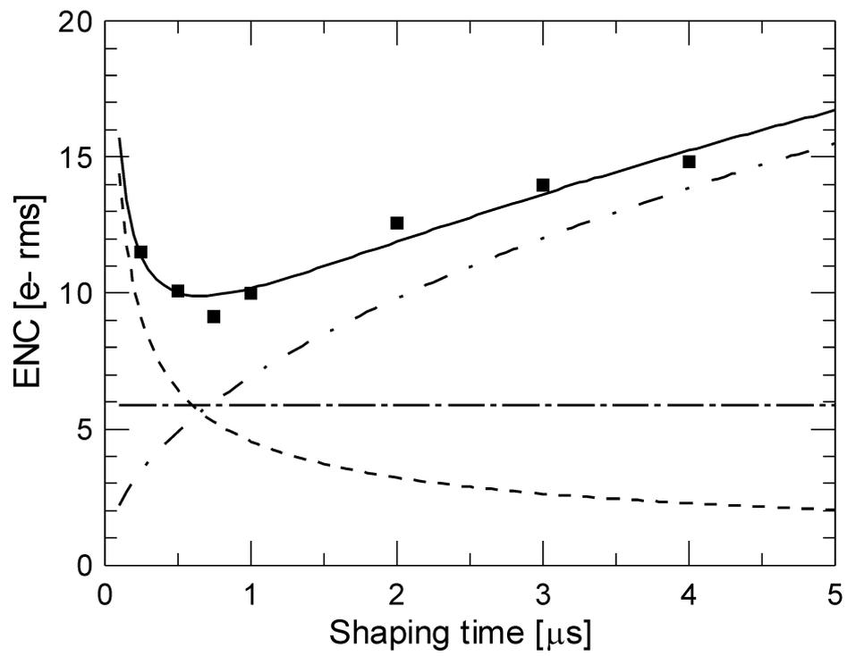
Fig. 11. ENC versus shaping time, measured at  $-10^{\circ}\text{C}$ .
