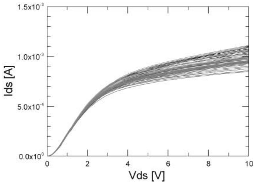
Fig. 6. Characteristics of the 77 on-chip JFETs.
