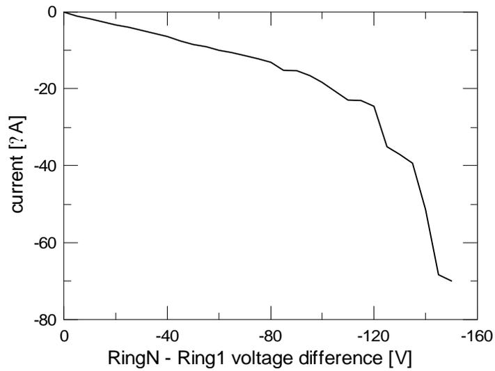
Fig. 4. Electrical characteristic of the integrated voltage divider implemented for the biasing of the SDD drift rings through only the application of voltages to the last and first rings.
