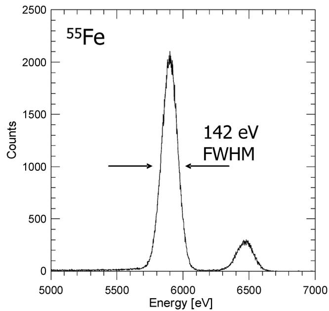
Fig. 10.  $^{55}\text{Fe}$  spectrum measured on a single unit of the array at  $-10^\circ\text{C}$  and using a shaping time of  $0.75\mu\text{s}$ .
