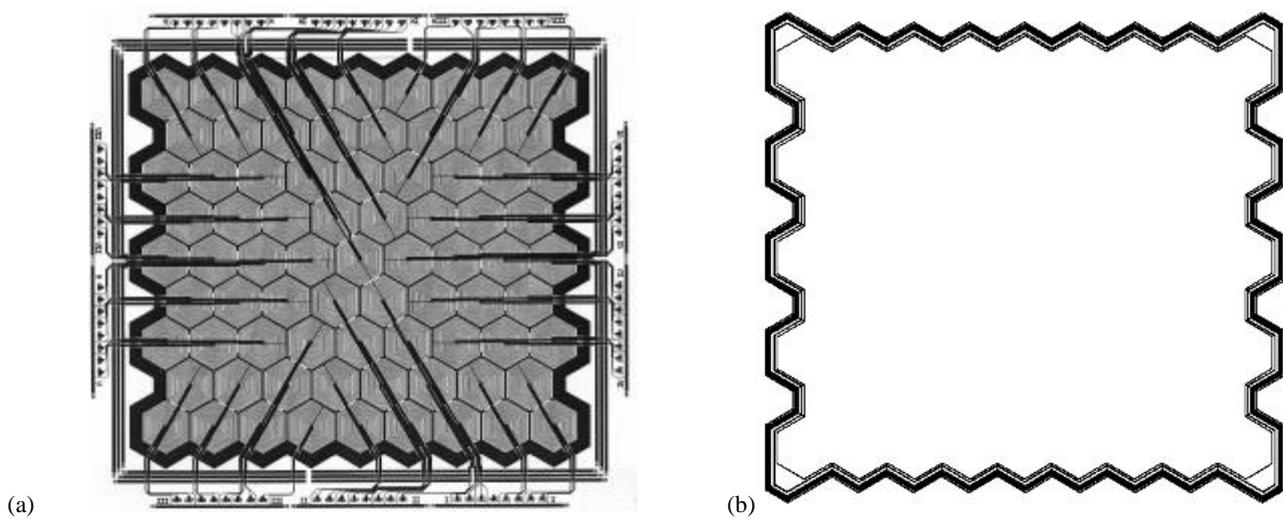
Fig. 1. Layout of the monolithic array of 77-SDDs. The detector side where the drift rings and the front-end JFET are integrated is shown in the figure (a). The entrance window for X-rays of scintillation photons is the opposite side of the detector (b).
