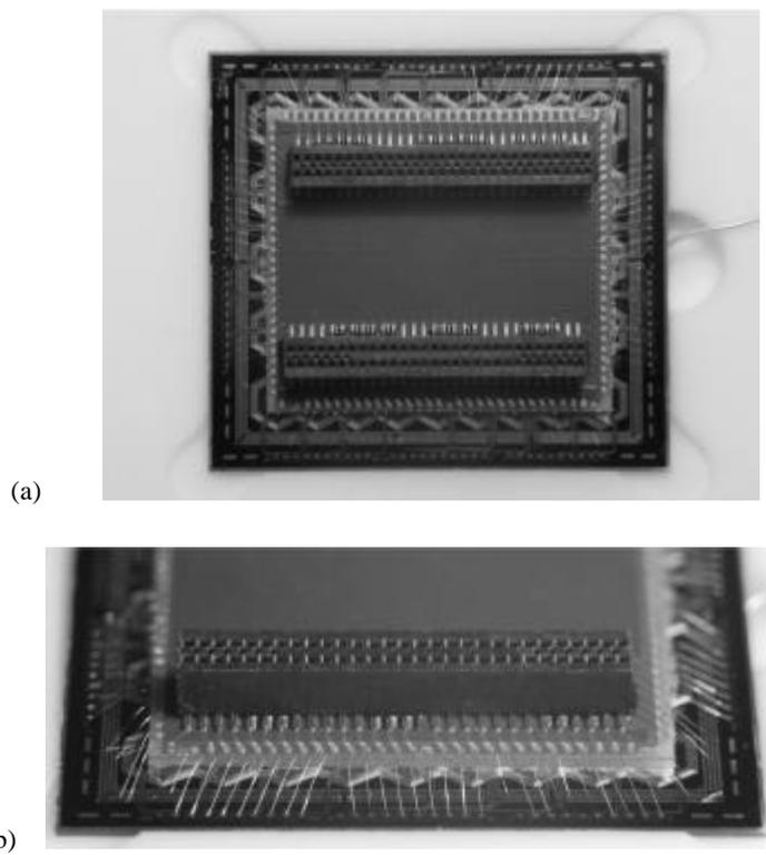
Fig. 2. (a) Mounting of the hybrid on the front side of the monolithic array. (b) Detail of the bonding connections.
