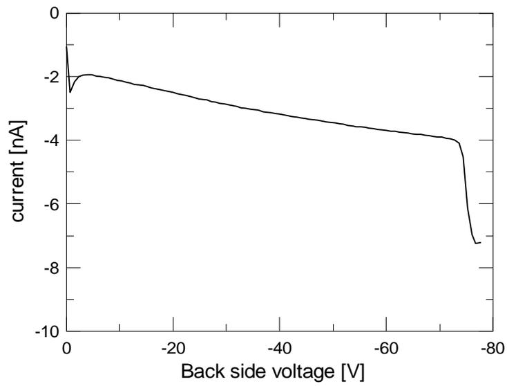
Fig. 3. Measurement of the leakage current on the back side of the detector, common to all units.
