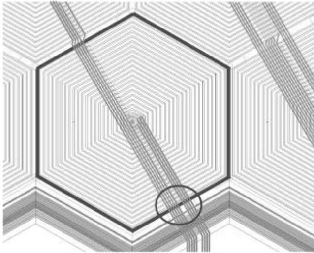
Fig. 5. Detail of the layout of a single SDD unit in the monolithic array. A region where the low-voltage bias lines are crossing the outermost ring (identified in the figure by the dark contour), biased at high voltage, is highlighted.
