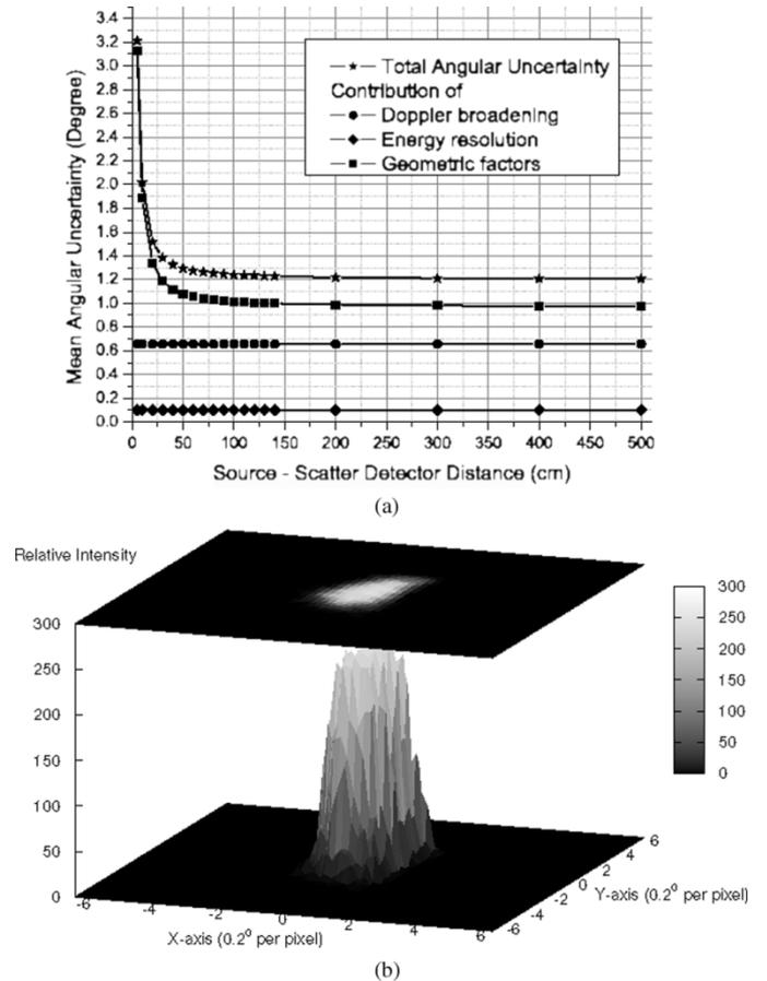
Fig. 9. Mean angular uncertainty calculated theoretically and the reconstructed image for a point source located 120 cm away from the first detector. The FWHM angular uncertainty calculated at this distance is within the expectation limits. (a) Expected angular uncertainty. (b) Reconstructed image.
