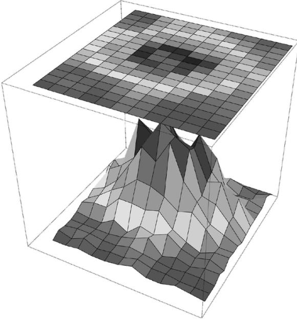
Fig. 3. x-y scan of a single SDD cell in  $400\ \mu\text{m}$  steps with  $662\ \text{keV}$  photons of  $^{137}\text{Cs}$  source.
