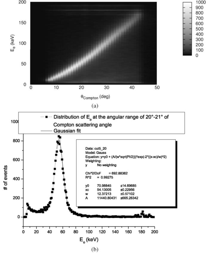
Fig. 7. The energy of the recoil electron measured in the SDD as a function of the Compton scattering angle and the distribution of the  $E_e$  at a fixed scattering angle. (a)  $E_e$  versus Compton scattering angle. (b) Distribution of  $E_e$  at  $20^\circ$ .
