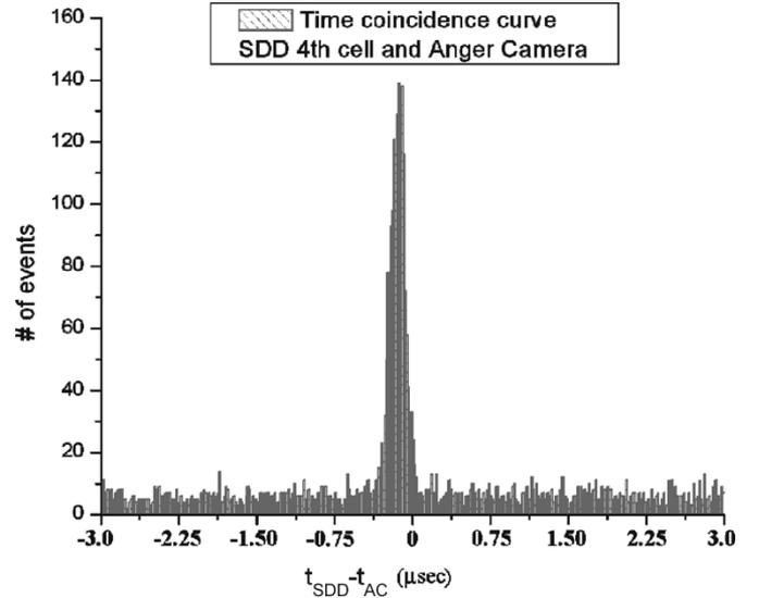
Fig. 5. Time coincidence curve for the coincident events occurring in the SDD and the Anger camera.
