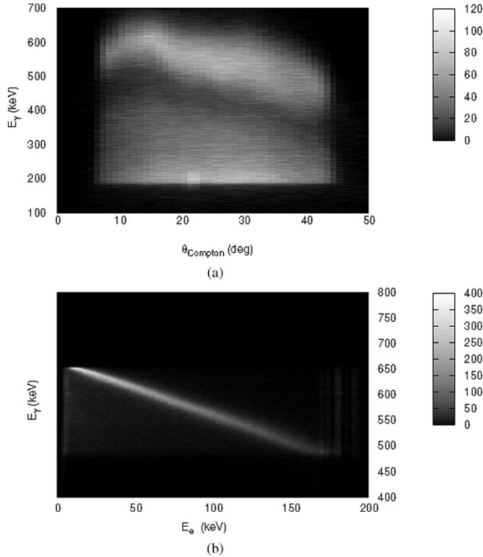
Fig. 8. The energy of the scattered photon measured in the Anger camera as a function of the Compton scattering angle and  $E_\gamma$  as a function of  $E_e$  where  $E_\gamma$  is calculated from the scattering angle. (a)  $E_\gamma$  versus Compton scattering angle. (b)  $E_\gamma$  vs  $E_e$ .
