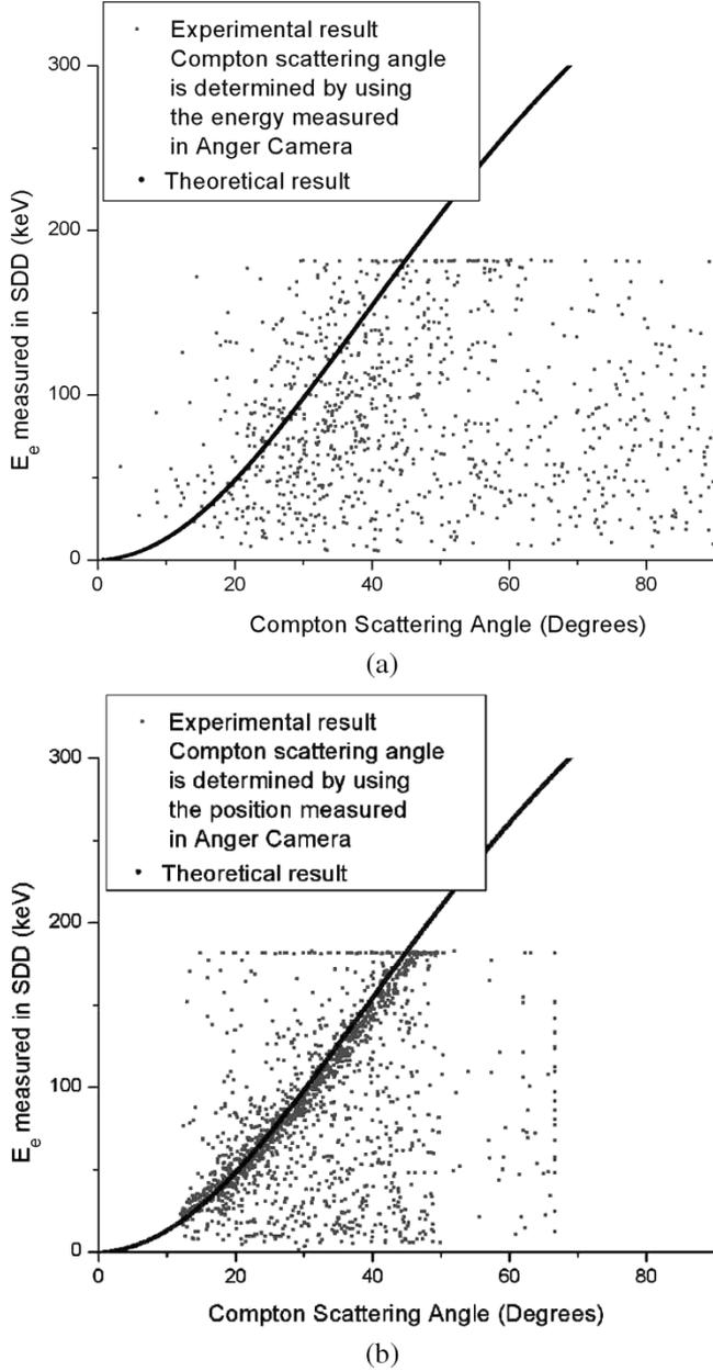
Fig. 6. The energy of the recoil electron measured in the SDD as a function of the Compton scattering angle which is calculated (a) using the energy measured in the Anger camera and (b) coordinate measured in the Anger camera.
