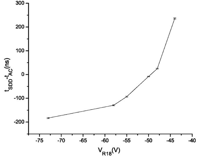
Fig. 4. The variation of the time stamp difference between the two detectors as a function of the drift field in the SDD.
