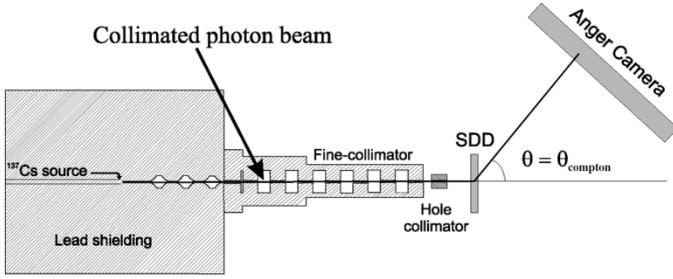
Fig. 2. The collimator setup for the 1-Ci  $^{137}\text{Cs}$  source.
