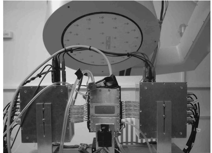
Fig. 1. The Compton camera test setup consisting of a silicon drift detector as a scatter detector and an Anger camera as an absorption detector.
