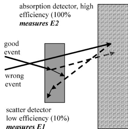
Fig. 9. Problem of misinterpretation of events using detectors in forward scattering geometry. Wrong events pass the first detector and are backscattered from the second detector.
