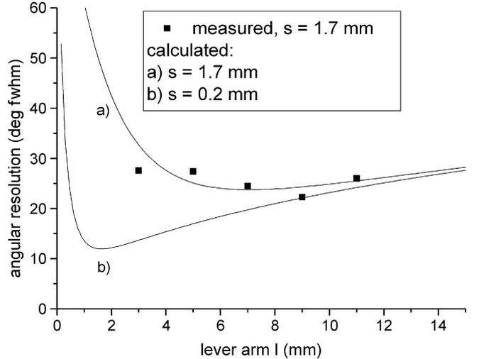
Fig. 4. Angular resolution in the direction of the mean ionization track with Kr-filling, 1.4 bar,  $s = 1.7$  mm. a) and b) calculated according to (1) for  $s = 1.7$  mm and 0.2 mm, respectively [2].
