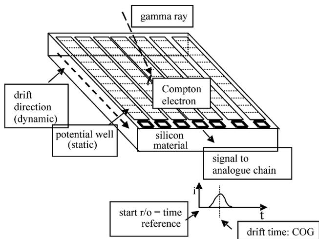
Fig. 7. Controlled Drift Detector (CDD, [9]), a Si-drift detector which generates its own start signal.
