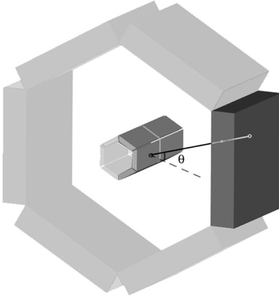
Fig. 5. Setup of Compton coincidence imaging system consisting of a smaller inner ring of a Si-stack and an outer one as absorption detector.
