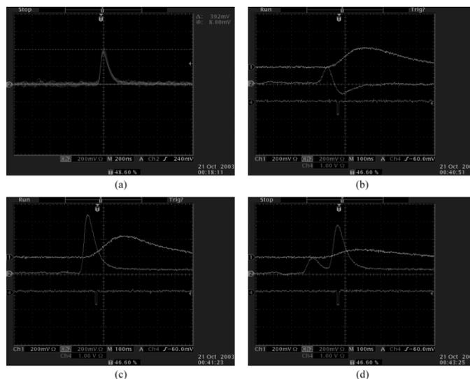
Fig. 10. Response to different ionization in the Si-drift chamber (middle trace). The corresponding signal of the Anger camera (upper trace) is shown in coincidence. The third trace is the coincidence gate. (a) Point-like ionization ( $^{55}\text{Fe}$ ). (b) Compton electron. (c) Compton electron. (d) Compton electron (double).
