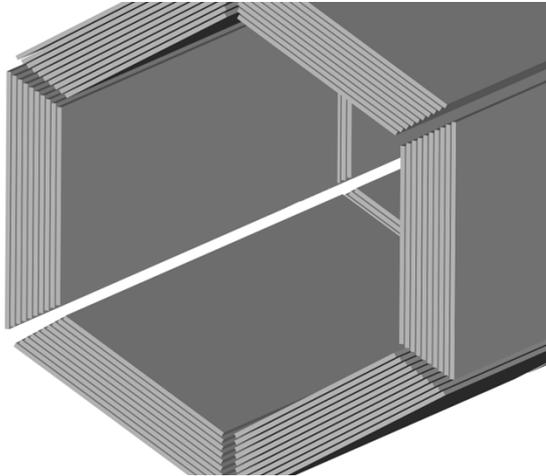
Fig. 6. Close-up of Si-stack. The individual Si drift detectors can be arranged in about 10 layers to have the ends free for connections of amplifiers and read-out.
