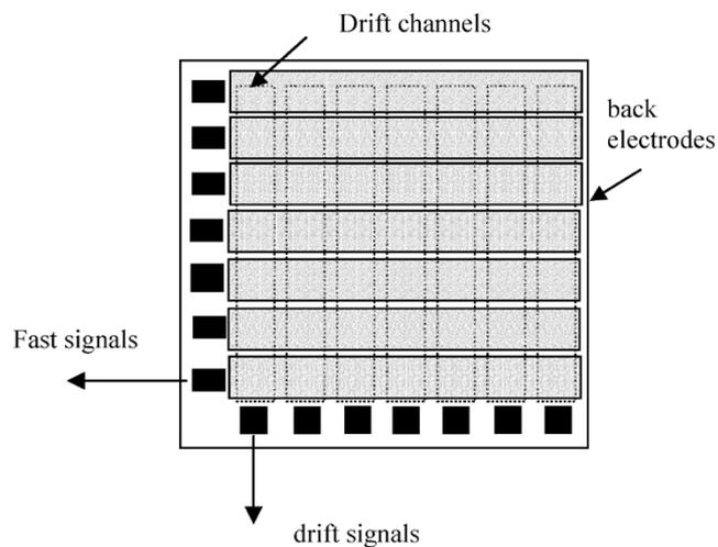
Fig. 8. Back-side read-out of Si drift detector.
