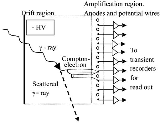
Fig. 3. Drift chamber (TEC) for measurement of Compton electron direction.
