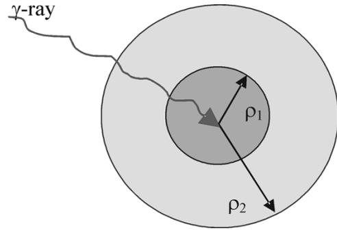
Fig. 1. Limits of position resolution for gamma rays. The range of secondary radiation is indicated. The smaller  $\rho_1$  could be due to the range of photo- or Compton-electrons, the larger  $\rho_2$  due to fluorescence or scattered radiation.
