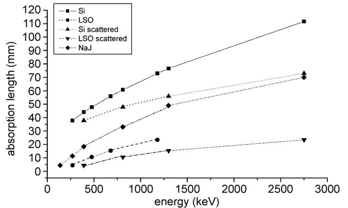
Fig. 2. Absorption length of primary and scattered radiation in detector material.
