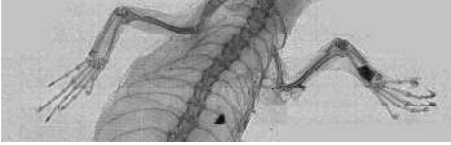
Fig. 2. X-ray radiographic image of a lizard acquired with a CDD operated at  $100kHz$  frame frequency ( $300K$ ). The image is obtained accumulating 150,000 frames. The energy of the incident beam was set to  $15keV$ . The darker the pixel in the gray scale, the lower the number of counts in the pixel.
