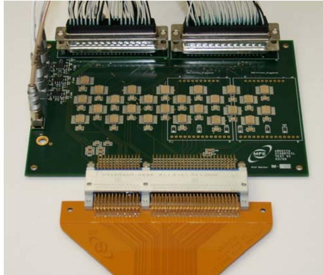
Figure 6: Prototype of the front-end board (top) connected with rigid-flex printed board (bottom).
