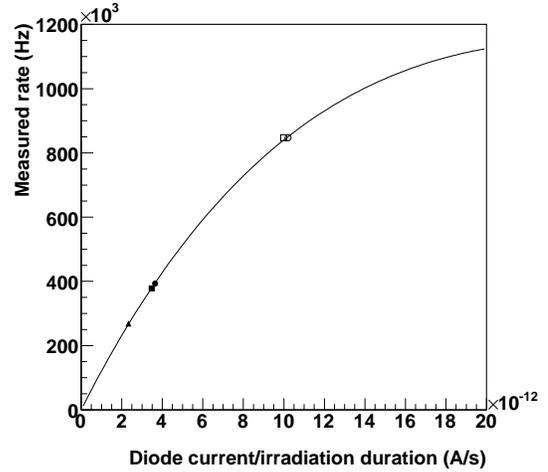
Fig. 7. Measured proton rate without corrections as a function of the ratio between diode leakage current and irradiations duration ( $i_D/t_{irr}$ ). The experimental measurements are superimposed to the fit with the function of Eq. 15.
