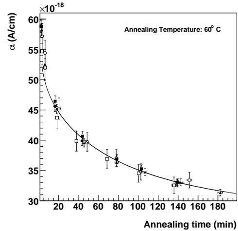
Fig. 8. Damage rate as a function of the annealing time at performed at 60° C.
