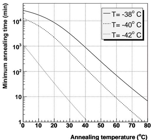
Fig. 10. Minimum annealing time required at different operation temperatures as a function of the temperature of annealing and at an integration time of  $128\mu\text{s}$ .
