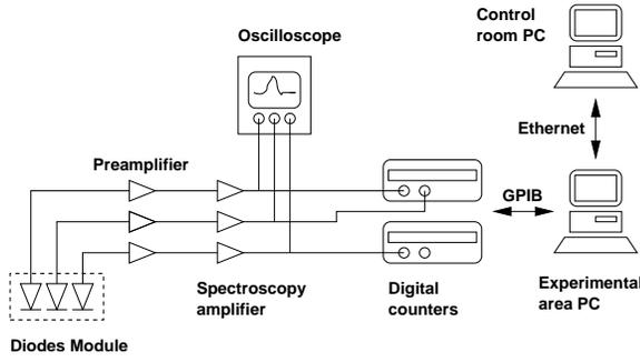
Fig. 6. Scheme of the DAQ system used for dosimetry.
