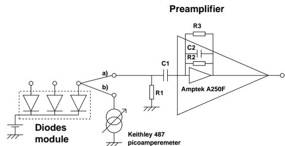
Fig. 5. Scheme of the biasing and preamplifying circuit. When the p+ contact of a diode is connected to the amplification chain according to the modality a) in the figure, the proton counting dosimetry can be performed, while when it is connected to the picoamperemeter in the modality b), the leakage current can be measured.
