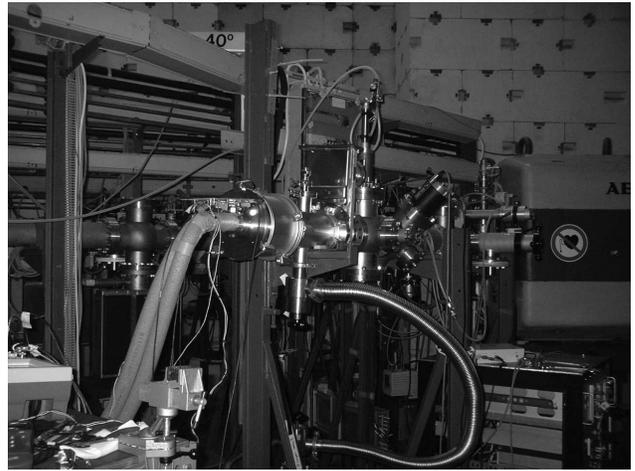
Fig. 4. A view of the experimental area as it was during the experiment. The cylinder was connected to the the accelerator vacuum pipe and the electronics, cooling and vacuum pump are inserted.
