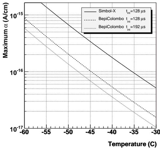
Fig. 1. Maximum current related damage rate allowing the target energy resolution for the Simbol-X and BepiColombo missions as a function of the operating temperature. The integration time ( $t_{int}$ ) related to the curves is reported.
