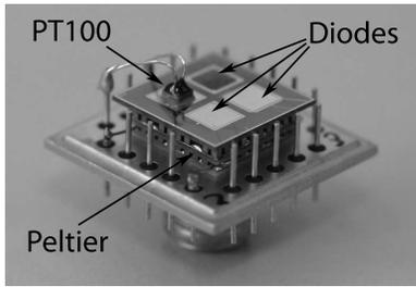
Fig. 2. Picture of a diode module. The main components are also indicated.
