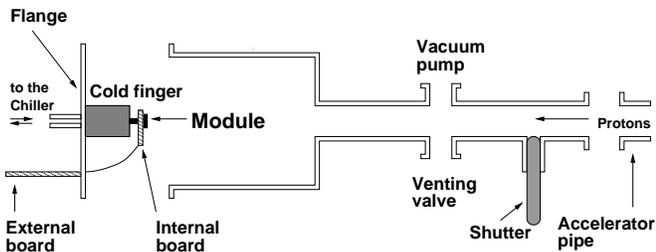
Fig. 3. Scheme of the vacuum cylinder and the flange.
