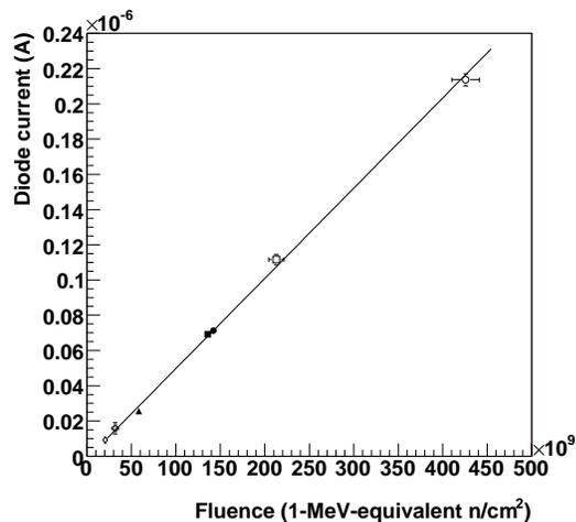
Fig. 9. The diode current measured at  $-50^{\circ}\text{C}$  (and normalized at  $20^{\circ}\text{C}$ ) as a function of the corrected fluence expressed in  $1\text{ MeV}$  equivalent neutrons/cm $^2$ . The fit is superimposed to the experimental measurement.
