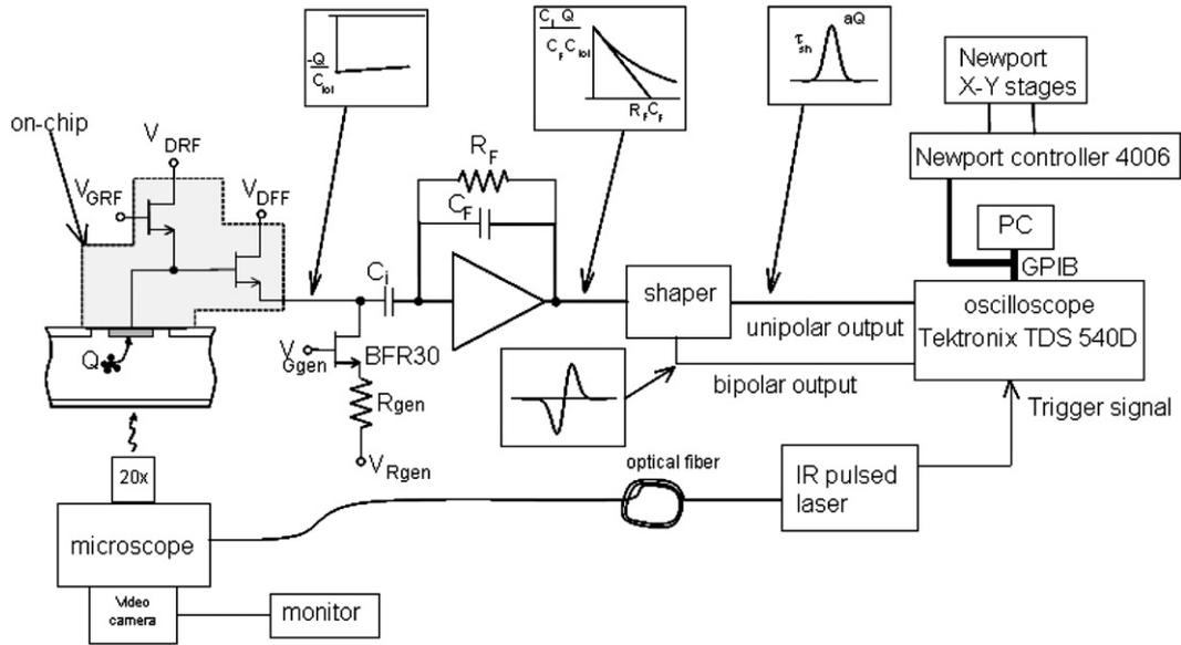
Fig. 2. Block diagram of the measurement setup and of the readout electronics.
