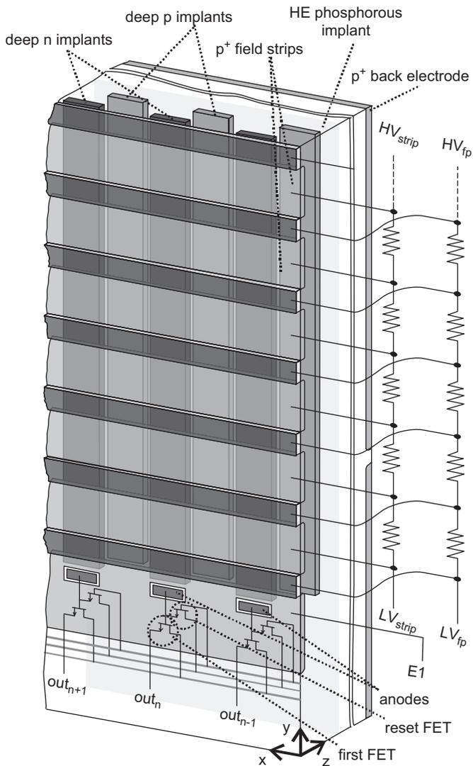
**Fig. 1.** Sketch of the architecture of the MLSDD prototype used in the present tests.
