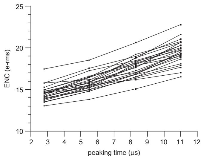
Fig. 5. Electronics noise measured for the 25 SDDs at  $-10$  °C and at different peaking times provided by the ASIC.
