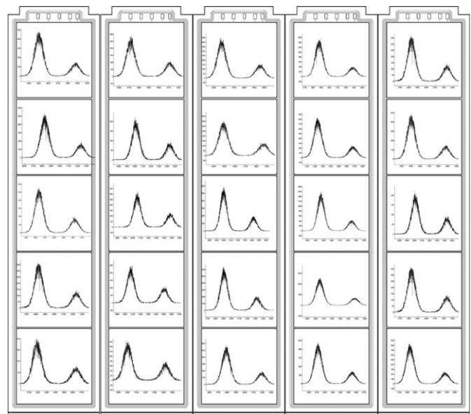
Fig. 4. Energy spectrum of a Fe<sup>55</sup> source measured at  $-10$  °C and with a peaking time of 5.5  $\mu$ s.
