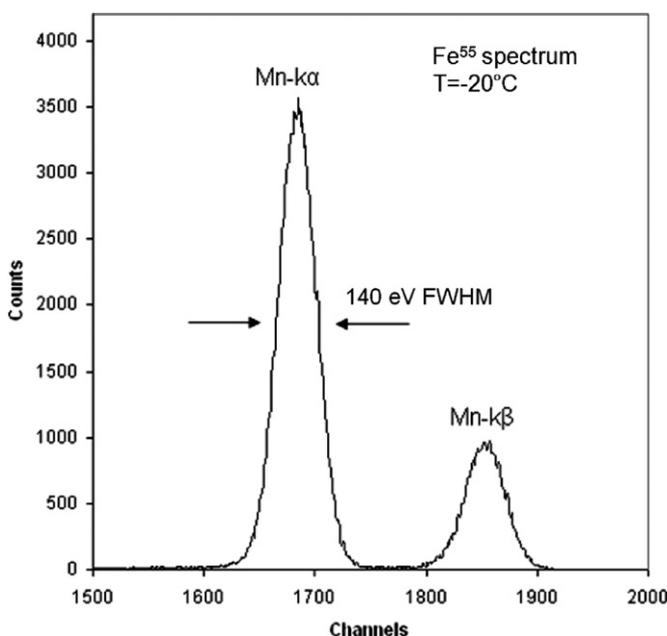
Fig. 3. Energy spectrum of a Fe<sup>55</sup> source measured at  $-20$  °C and a shaping time of 2  $\mu$ s.
