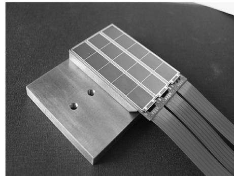
Fig. 2. Photograph of the assembly of 3 monolithic arrays of SDDs.
