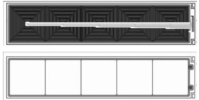
Fig. 1. Layout of the array of SDDs. On the lower section, the side where the scintillator is read out is shown while on the upper side the detector side with the drift rings and the on-chip JFET is shown.
