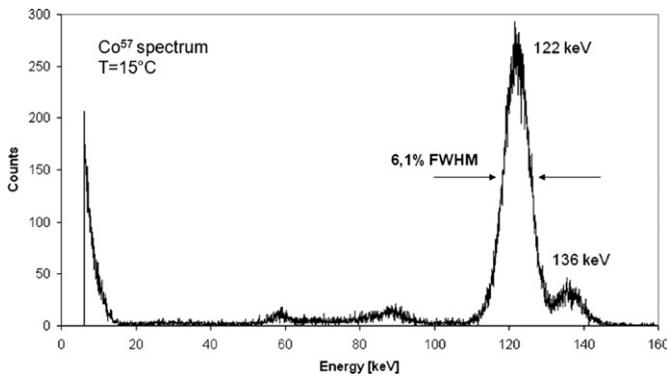
**Fig. 6.** Energy spectrum of a  $\text{Co}^{57}$  source measured at  $+15\text{ }^{\circ}\text{C}$  with a 10 mm thick CsI(Tl) scintillator coupled to the SDD unit. The shaping time of the measurement is 12  $\mu\text{s}$ .
