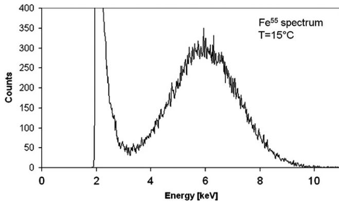
**Fig. 7.** Energy spectrum of a  $\text{Fe}^{55}$  source measured at  $+15\text{ }^{\circ}\text{C}$  with the CsI(Tl) scintillator coupled to the SDD unit. The shaping time of the measurement is 2  $\mu\text{s}$ .
