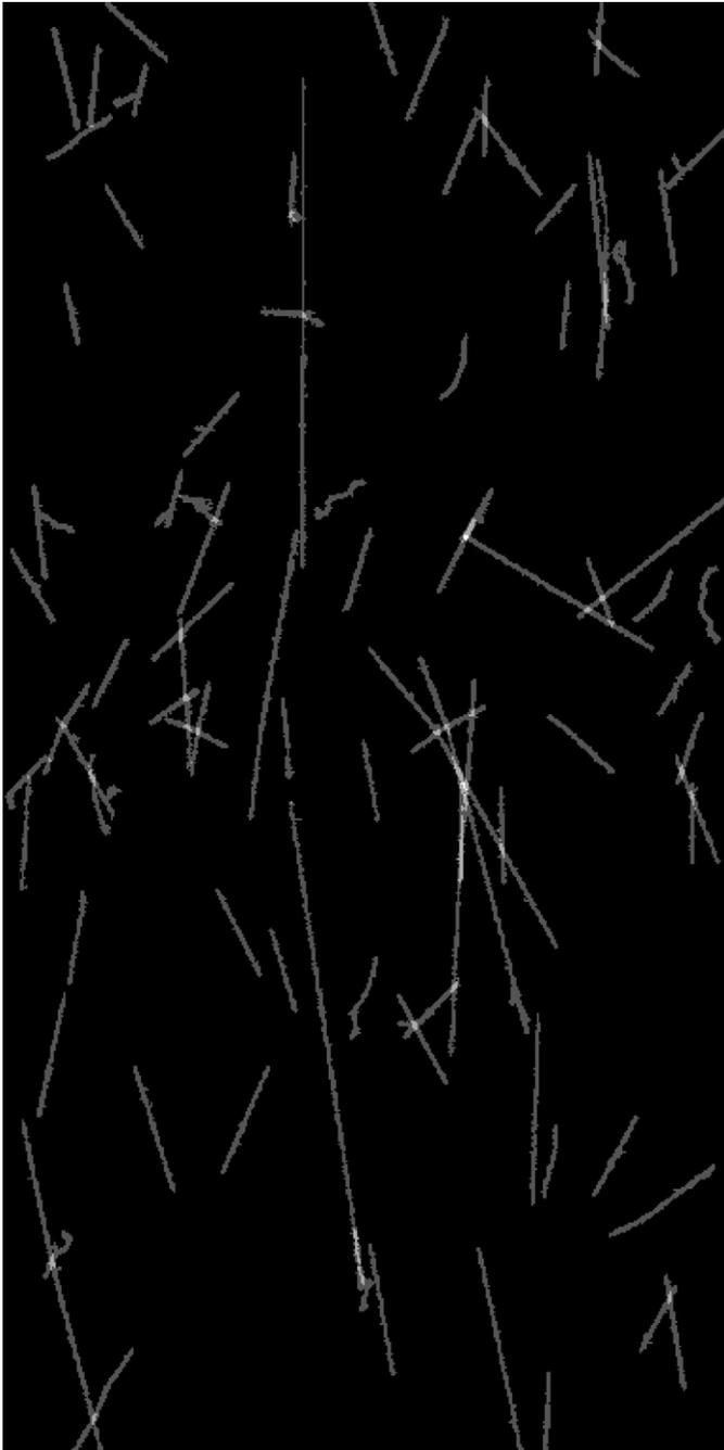
**Fig. 12.** Selected prominent MIP tracks measured in dark field with an eROSITA PNCCD detector in full frame mode ( $384 \times 768$  pixels).
