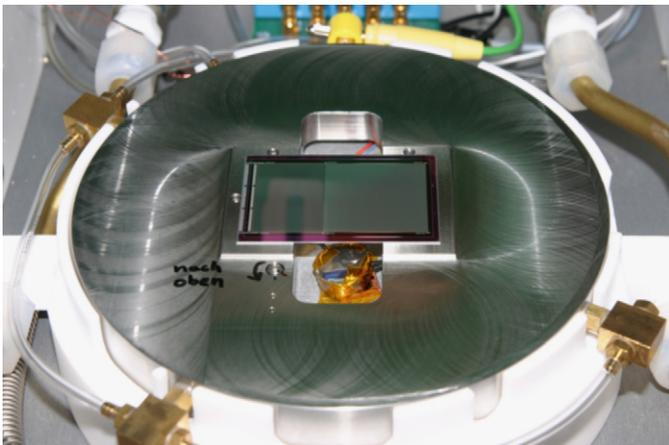
**Fig. 2.** An eROSITA-PNCCD mounted on the chuck which can be cooled with liquid nitrogen. Underneath the CCD one of the  $^{55}\text{Fe}$ -sources for back side illumination can be seen.
