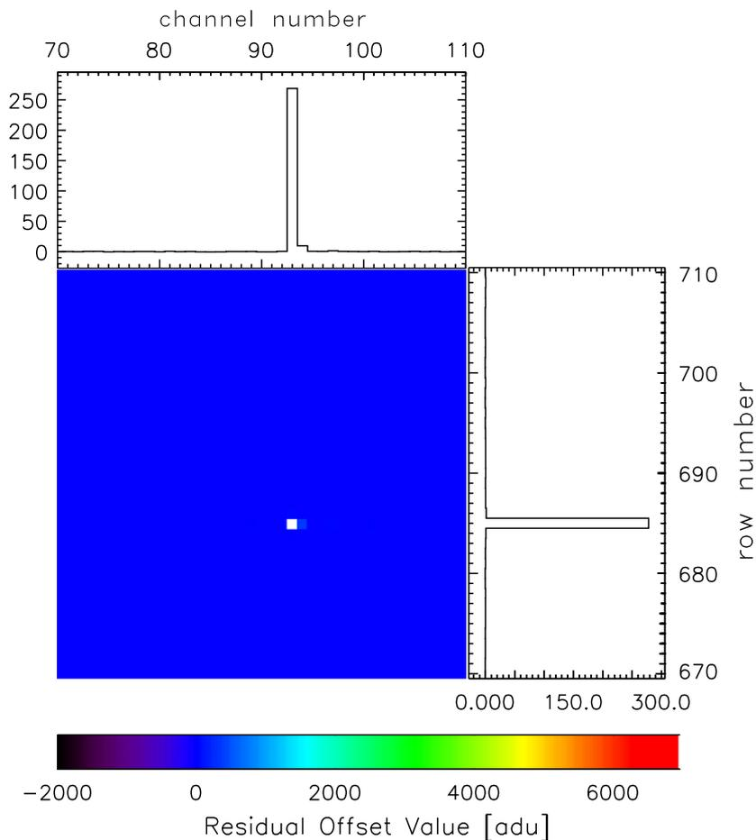
Fig. 5. This residual offset map shows a bright pixel in channel 93 and row 685.
