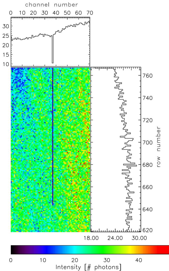
**Fig. 6.** Part of an intensity image showing a non-transferring-pixel. Behind the non-transferring-pixel the intensity is nearly zero.
