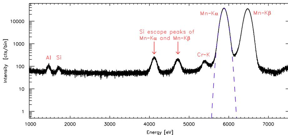
**Fig. 3.** This plot shows an  $^{55}\text{Fe}$ -spectrum measured with a PNCCD at  $-70^\circ\text{C}$  in the Cold Chuck Probe Station. The FWHM at 5.9 keV is 157 eV. In addition to the Mn-K $\alpha$  and Mn-K $\beta$  peaks, both Si escape peaks can be seen. The Al, Si and Cr-K lines are due to the setup. X-rays enter the CCD from the front and the back side in this setup resulting in an increased fraction of partial events.
