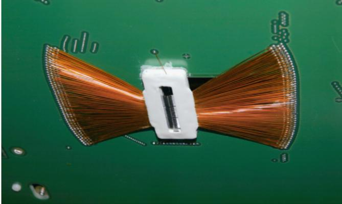
**Fig. 1.** The probe card with the needles mounted on it. Through the needle contacts all operating voltages are supplied and the CCD signals are read out.
