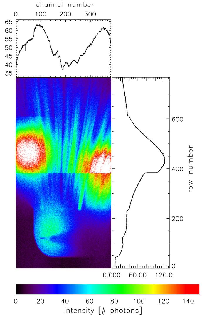
**Fig. 4.** Intensity map of a Cold Chuck Probe Station measurement showing the inhomogeneous illumination caused by the needles.
