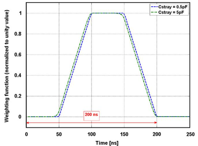
Fig. 6. Simulated weighing function for FCF. Two different stray capacitance values are considered. In both cases, simulations show a well defined trapezoidal behavior. During the central flattop the charges generated by XFEL pulses are collected into the DePFET internal gate.
