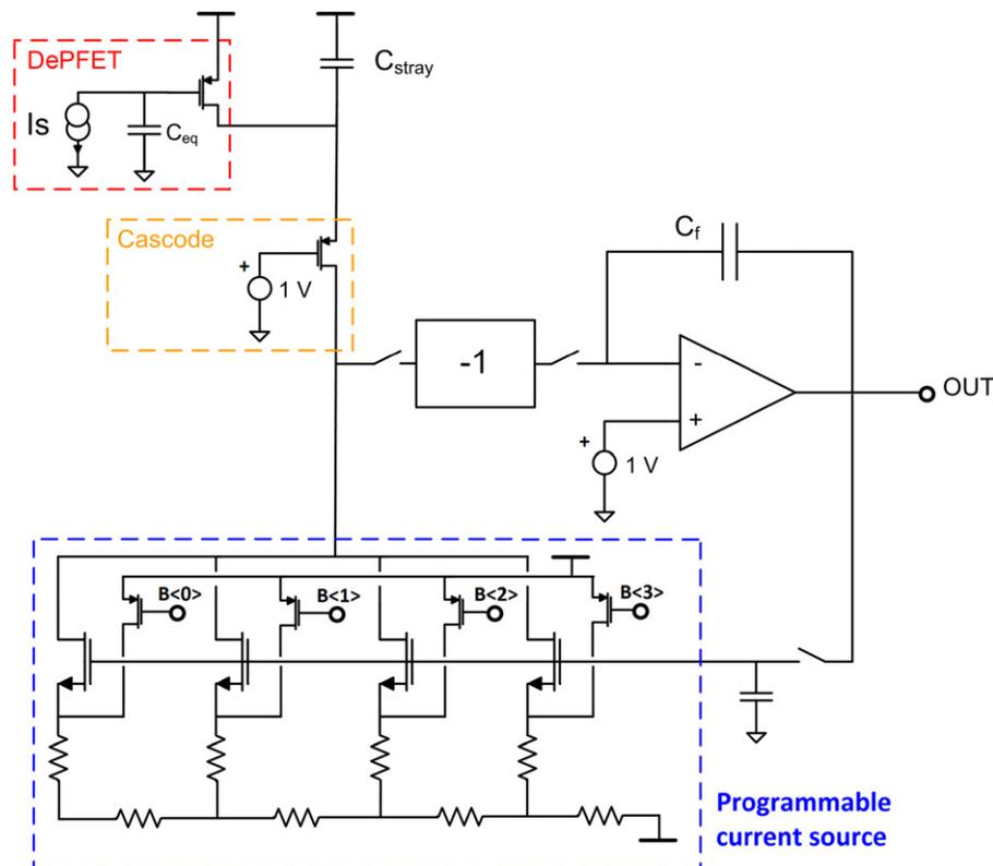
**Fig. 2.** The programmable current source principle structure. Once the active branches are selected by proper setting of the bits, a fine regulation of the current is obtained working on the gate voltage of these branches. This is done before every macro bunch.
