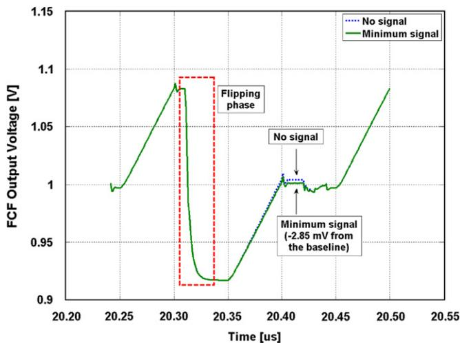
Fig. 5. Comparison between the output voltage without incoming photons and the output voltage corresponding to a single photon at 1 keV. The corresponding voltage variation is 2.85 mV, a value that fulfill well the requirements imposed by the subsequent ADC binning.
