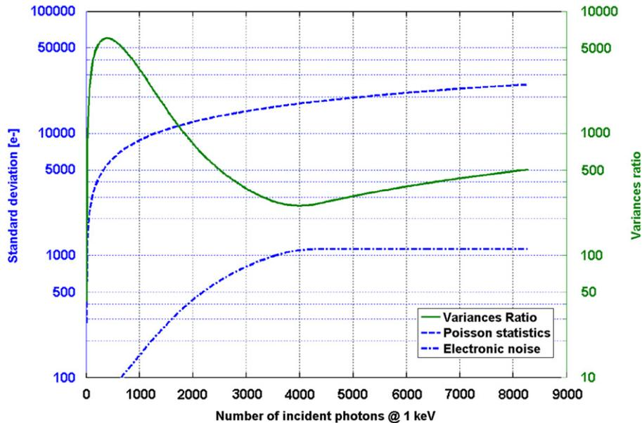
**Fig. 7.** Standard deviation of the Poisson distribution for the incoming photons and of the electronic noise introduced by the FCF in the whole dynamic range. The ratio of the square of these two parameters is also shown; this ratio increases at higher signal levels and remains greater than unity, and therefore the total noise is always dominated by the photon statistics, even if the electronics noise contribution increases due to the compressive behavior of the DSSC.
