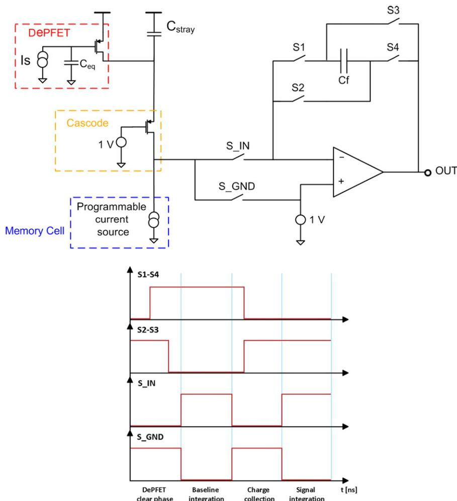
**Fig. 1.** Schematic representation of Flip Capacitor Filter (FCF) analog filter. In this architecture only one operational amplifier is used, and the desired trapezoidal weighting function is here achieved by flipping the feedback capacitor  $C_f$  by mean of four switches [S1 ÷ S4]. The timing diagram of signals controlling the switches is shown.
