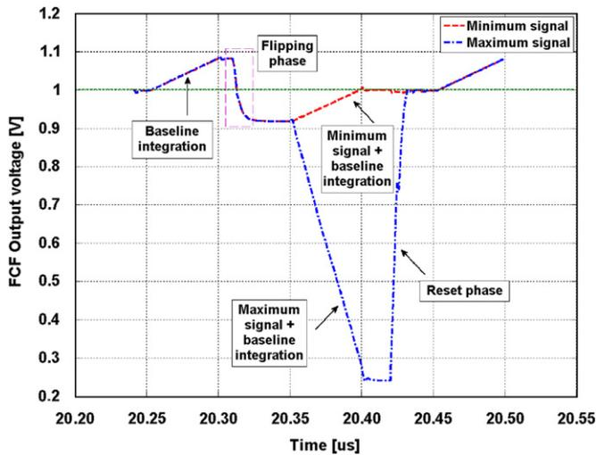
Fig. 4. Output filter voltage swing for minimum and maximum signals at 5 MHz timing operation. Double correlated sampling is simulated with a baseline of  $-3 \mu\text{A}$ , and the flipping phase is highlighted.
