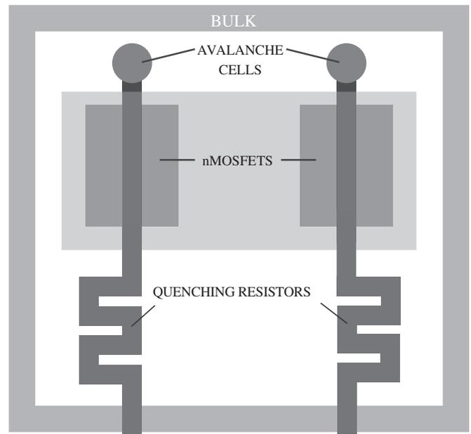
Fig. 13. Schematic top view of a test structure with cells of  $9\mu\text{m}$  diameter for investigating the dark current contribution of single readout cells. The bulk contact is the most positive one such that electrons from the surrounding area outside the cells do not contribute to dark counts.
