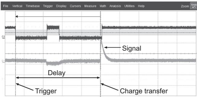
Fig. 11. Snapshot from a digital oscilloscope illustrating the principle of the time-correlated measurement. Refer to text for the details.
