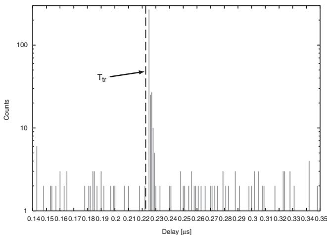
Fig. 12. Measurement of the time correlation between charge shifting and avalanche signal. Asymmetry in the time distribution is due to the fact that the avalanche signals are correlated with the charge transfer ( $T_{tr}$ ) and cannot occur ahead of this.
