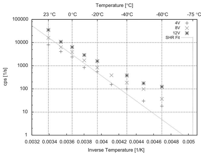
**Fig. 14.** Dark rate dependence on temperature and overbias for a single avalanche cell with  $9\ \mu\text{m}$  diameter. Exponential decay down to 30 counts/s has been measured. The data points follow SHR generation (linear fit at 8 V overbias) only for the higher temperature regime with a progressive departure of the experimental data from the model at lower temperatures.
