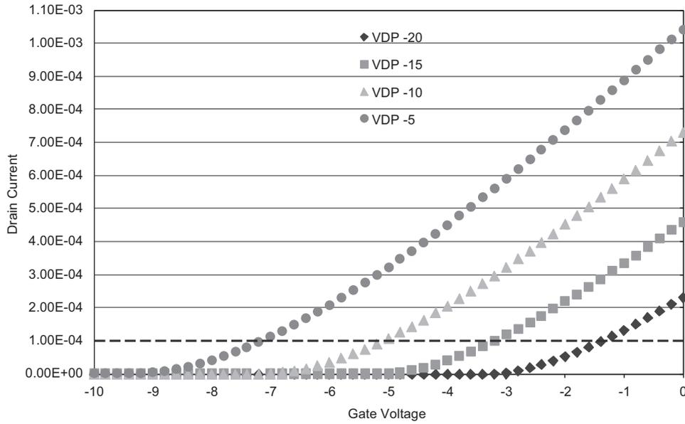
**Fig. 7.** Input characteristics of the front-end transistor used as the first amplification stage in source-follower configuration with constant current load. The strong steering power of the deep p-doped well is accounted for by the modulation in threshold voltage of over 10 V. The constant bias current level of 100  $\mu$ A is indicated by the dashed line.
