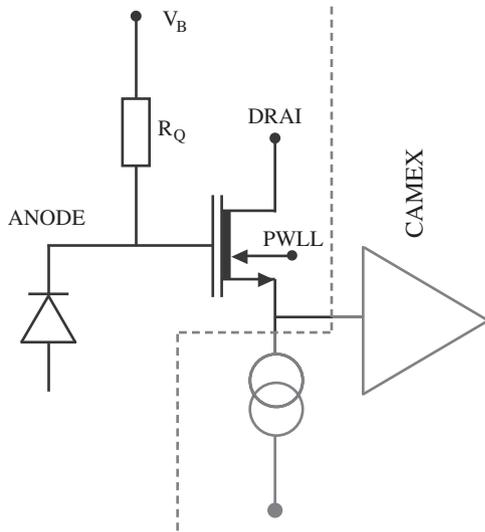
**Fig. 8.** Schematic diagram showing the readout chain of an arbitrary CCD column. The front end transistor is working as source follower and coupled to the CAMEX amplifier.
