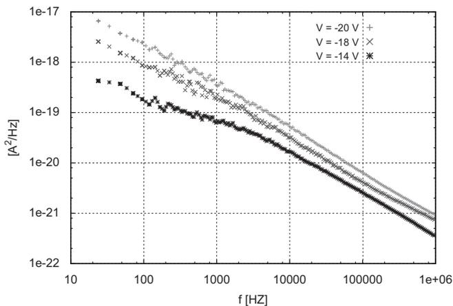
**Fig. 6.** Power spectral densities of the front-end transistor used as first amplifier. The curves correspond to three different voltages of the embedding p-type well.
