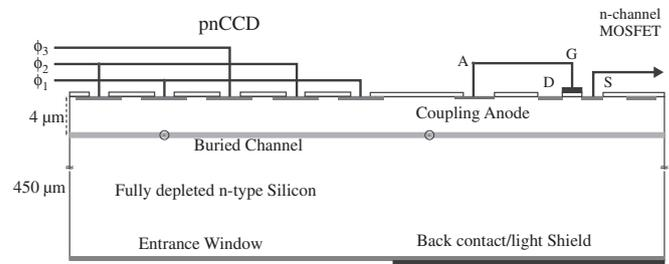
**Fig. 3.** Cross-section view of a simplified device. The high-field implants and the quenching resistor are omitted to test basic functionality and perform spectroscopic measurements.
