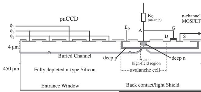
**Fig. 2.** Cross-section view along the dashed line in Fig. 1. The transfer direction for signal electrons is from left to right.
