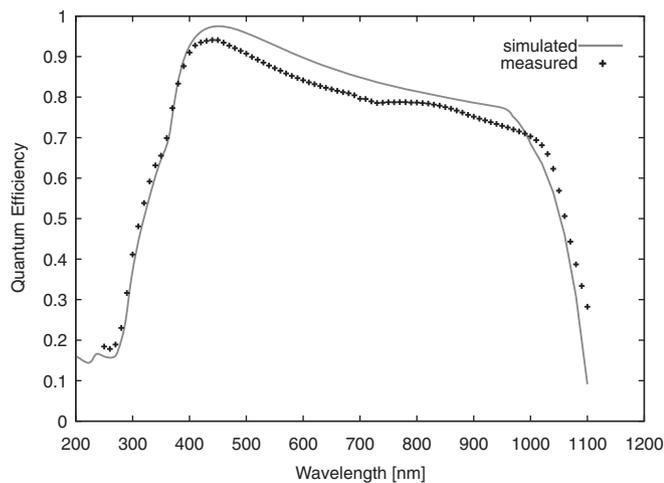
**Fig. 15.** Simulated (solid curve) and measured (points) quantum efficiency of avalanche pnCCD entrance window with anti-reflective-coating.
