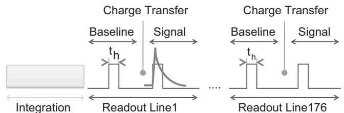
**Fig. 10.** Time structure of a whole frame cycle. After the charge collection time, the 132 pixels of the first CCD row are processed in parallel. A single sample placed immediately after the charge shift is enough to capture most of the fast decaying avalanche pulse, while another one is needed to set the baseline of the system.
