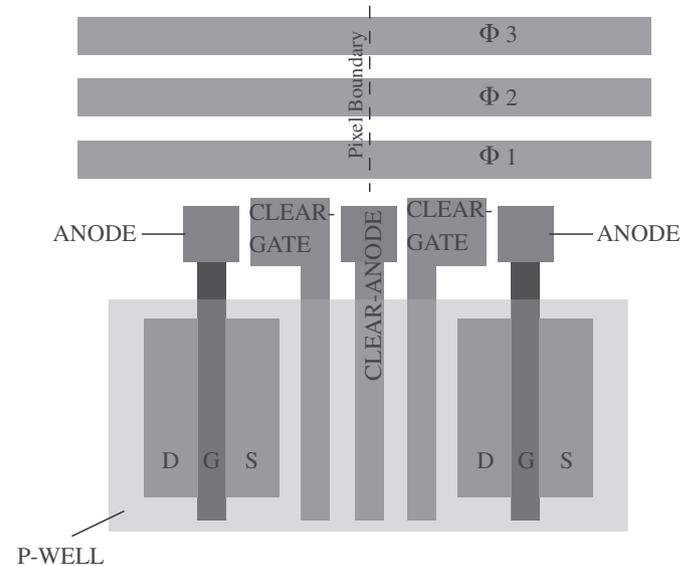
**Fig. 4.** Schematic top view showing the readout region of a simplified pnCCD produced in the new avalanche technology. Charge transfer direction is top down. The collecting anode is coupled to the transistor gate, one transistor per column. Two readout anodes share a common clear contact located in between.
