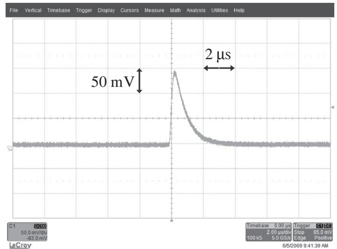
**Fig. 9.** Pulse waveform of an avalanche generated by a dark electron.
