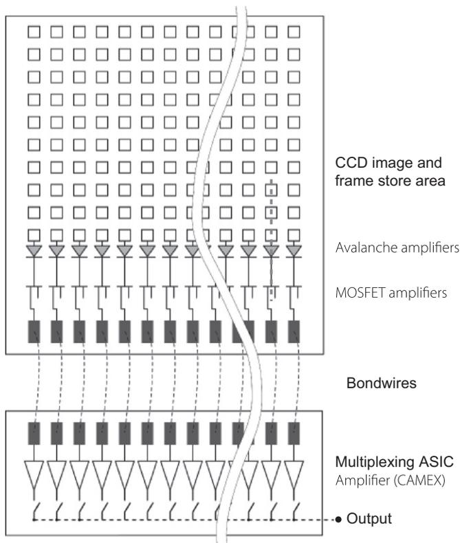
**Fig. 1.** Schematic picture of an avalanche amplifying pnCCD. Every column in the sensitive region (CCD image and frame store area) is coupled to an avalanche diode operated in Geiger mode. The signal is buffered by an on-chip source-follower wire bonded to an ASIC amplifier.
